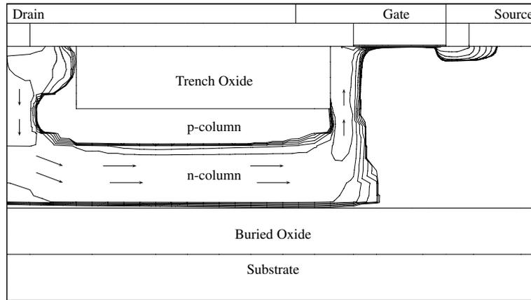
Fig. 2. Current distribution of a SJ SOI-LDMOSFET with a trench oxide at  $V_{GS} = 15$  V and  $V_{DS} = 20$  V. The arrows show the current flow in the drift region.
