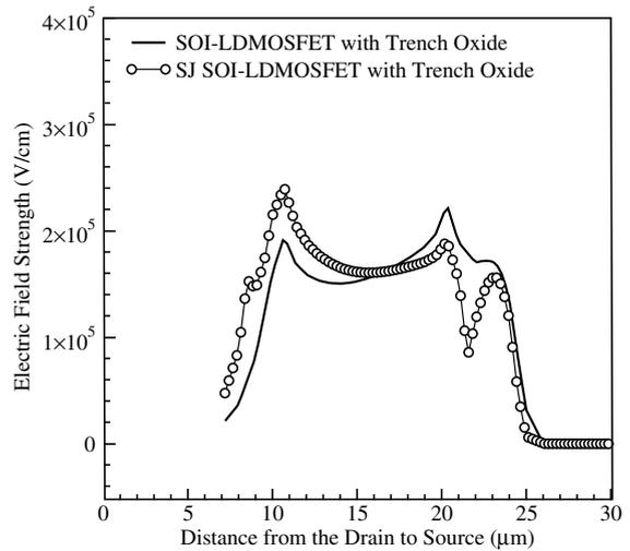
Fig. 7. Comparison of the electric field strength at the bottom of the trench oxide between the SOI-LDMOSFET and the SJ SOI-LDMOSFET. Both structures have a trench oxide in the drift region with  $L_d = 13.0 \mu\text{m}$ .
