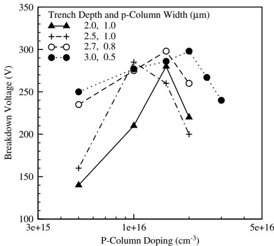
Fig. 9. BV versus  $p$ -column doping of the SJ SOI-LDMOSFETs with trench oxide which have  $L_d = 13.0 \mu\text{m}$  and  $N_D = 6.0 \times 10^{15} \text{cm}^{-3}$ .
