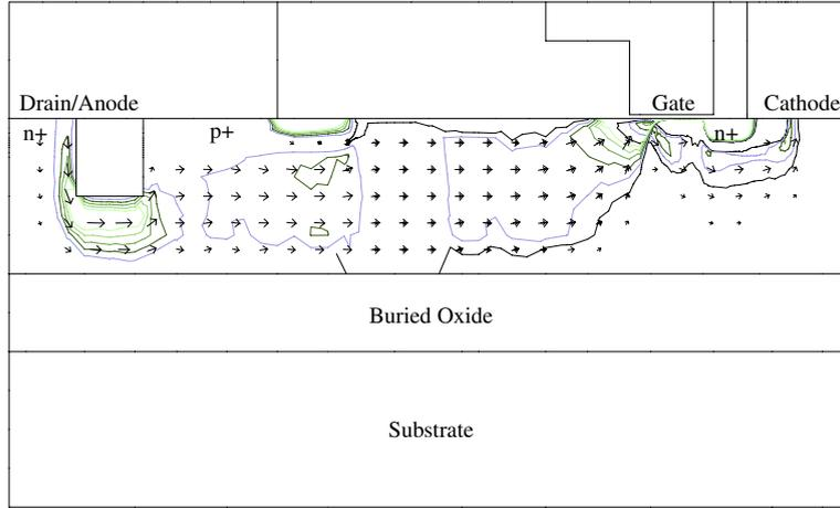
Fig. 4. Current flow in the proposed SA-LIGBT at  $V_G = 12$  V and  $V_A = 10$  V.
