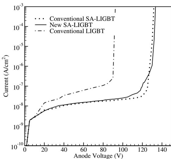
Fig. 11. BV comparison of the conventional SOI-LIGBT, and the conventional and proposed SOI SA-LIGBTs. Lower leakage currents can be seen at the SA-LIGBTs.
