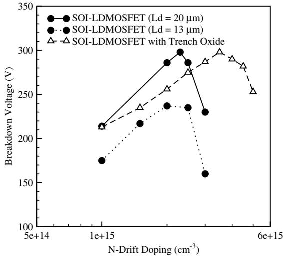
Fig. 8. BV versus  $n$ -drift doping of the conventional SOI-LDMOSFETs and SOI-LDMOSFET with trench oxide (trench depth = 2.7  $\mu\text{m}$  and  $L_d = 13.0 \mu\text{m}$ ).
