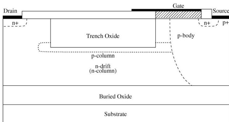
Fig. 1. Schematics of the SJ SOI-LDMOSFET with a trench oxide in the drift region.
