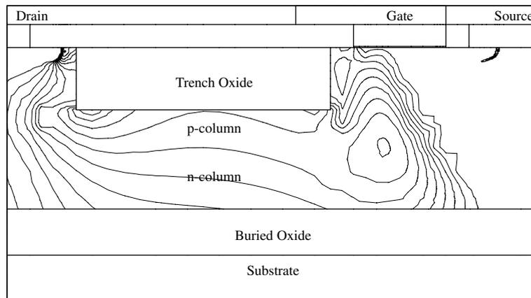
Fig. 6. Electric field distribution of a SJ SOI-LDMOSFET which has a trench oxide in the drift region at  $V_{DS} = 300 \text{ V}$ .
