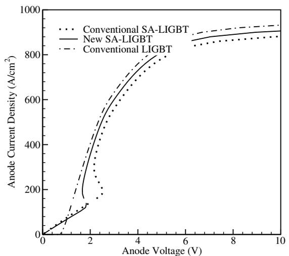
Fig. 12.  $I-V$  comparison of the conventional SOI-LIGBT and the conventional and proposed SOI SA-LIGBTs. A reduced snap-back voltage of the proposed device can be seen.
