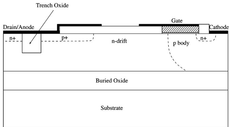
Fig. 3. Schematic structure of the proposed SOI SA-LIGBT with a trench oxide at the drain/anode.
