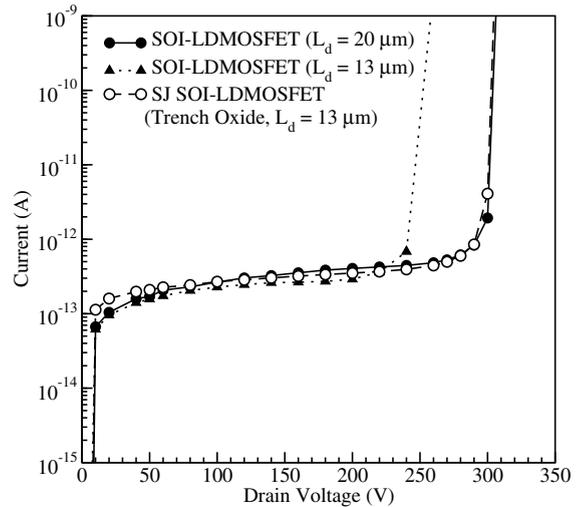
Fig. 5. Comparison of the BV of the conventional SOI-LDMOSFETs ( $L_d = 20.0$   $\mu\text{m}$  and  $13.0$   $\mu\text{m}$ ) and the SJ SOI-LDMOSFET with trench oxide ( $L_d = 13.0$   $\mu\text{m}$ ).  $N_D$  of conventional devices are  $2.3 \times 10^{15}$   $\text{cm}^{-3}$  (at  $L_d = 20.0$   $\mu\text{m}$ ) and  $3.5 \times 10^{15}$   $\text{cm}^{-3}$  (at  $L_d = 13.0$   $\mu\text{m}$ ), respectively, and  $6.0 \times 10^{15}$   $\text{cm}^{-3}$  of the SJ SOI-LDMOSFET.
