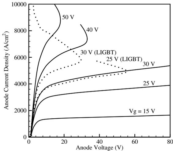
Fig. 13. On-state characteristics of the proposed SOI SA-LIGBT and a conventional SOI-LIGBT. The considerable improvement of the latch-up can be seen.
