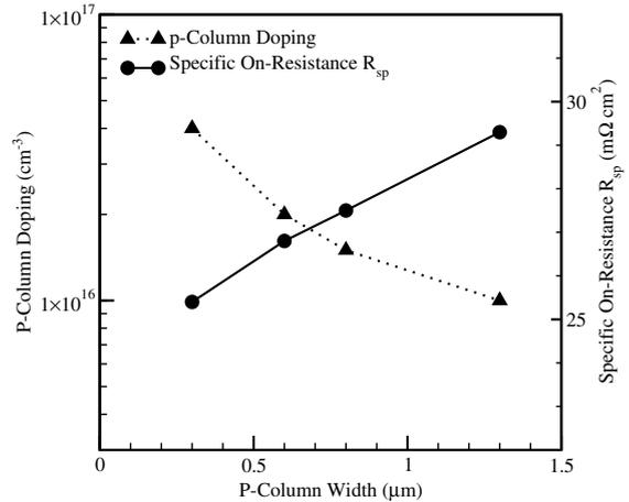
Fig. 10.  $p$ -column doping and  $R_{SP}$  versus  $p$ -column width of the SJ SOI-LDMOSFET which has a trench oxide.
