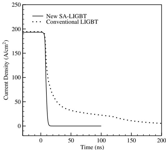
Fig. 14. Turn-off characteristics of the proposed SOI SA-LIGBT and a conventional SOI-LIGBT at the anode current density  $190 \text{ A/cm}^2$ ,  $V_A = 50 \text{ V}$ , and  $V_G = 12 \text{ V}$ . The tail current does not exist for the SOI SA-LIGBT.
