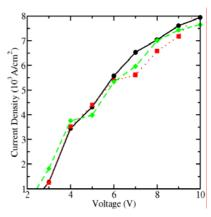
cover boundary and interface effects. Molecules have been modeled as particle-resevoirs mirroring the molecule size. Our attempts (Figure) to reproduce the current-voltage characteristics of amorphous ZnPc:0.3%F<sub>4</sub>TCNQ measured by (3) for 5, 10 and 15 % Gaussian spacial disorder show that this approach establishes a promising way of simulating the effects of morphology, doping and carrier concentration, all on a common footing.
