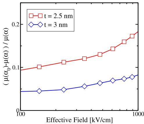
**Fig. 6** Relative correction to the channel mobility due to the thickness-dependence of the nonparabolicity parameter in the unprimed subbands.
