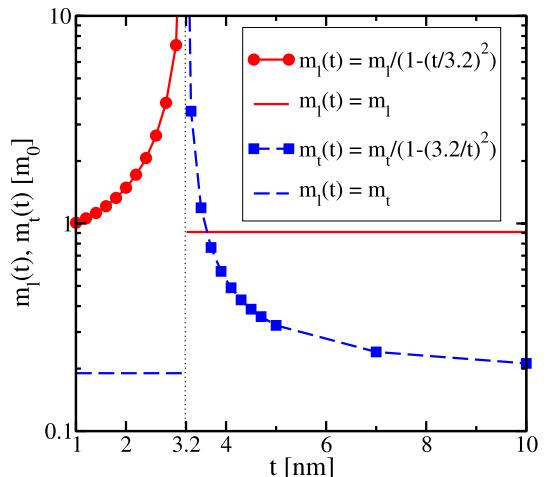
**Fig. 5** Dependence of the effective masses on the Si film thickness  $t$  at the minimum of the first primed subband
