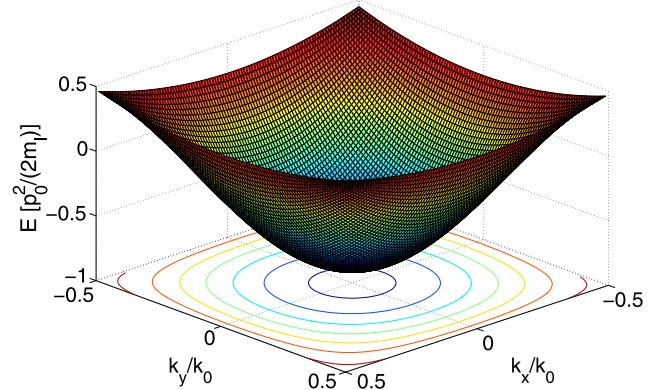
**Fig. 1** Dispersion relation (4) for the first unprimed subband ( $p_0 = \hbar k_0$ ), for (001) Si film with thickness  $t = 5 \text{ nm}$
