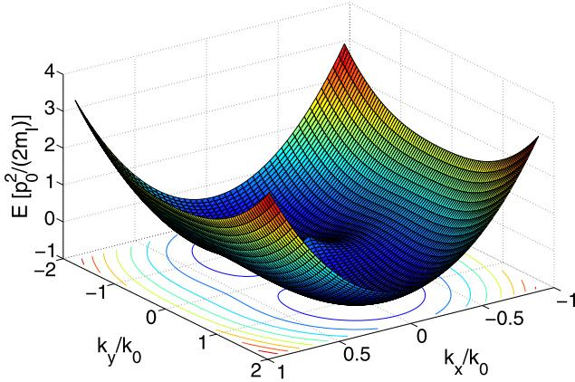
**Fig. 3** Dispersion relation for the first primed subband for (100) Si film with thickness  $t = 5$  nm
