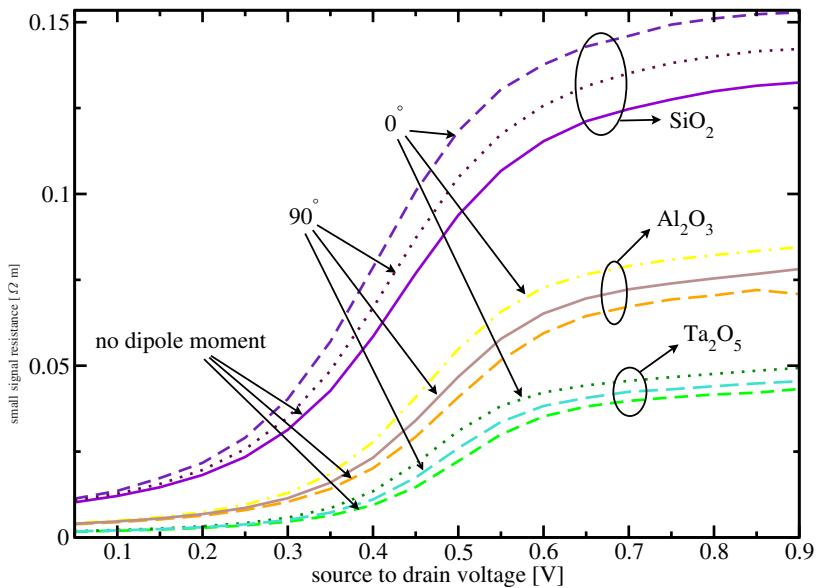
**Fig. 10.** Small signal resistance for  $\text{SiO}_2$ ,  $\text{Al}_2\text{O}_3$ , and  $\text{Ta}_2\text{O}_5$  calculated without dipole moment, angle  $0^\circ$  (perpendicular to surface), and angle  $90^\circ$  (parallel to surface) at bound state (biotin-streptavidin) for 10 nm average distance.
