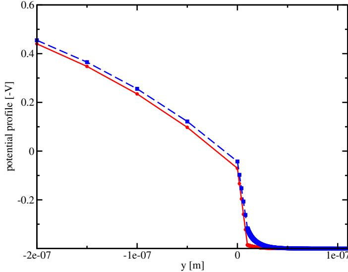
**Fig. 3.** Potential profile at the interface (from left to right: semiconductor, oxide, solute). The dashed line shows the profile, when biotin and streptavidin are attached to the surface (for 10 nm density), while the full line shows the potential with water and salt only.
