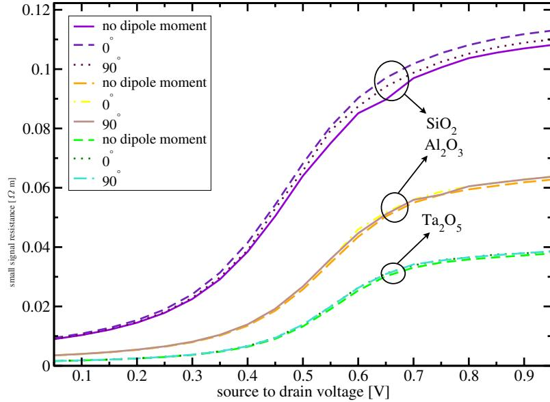
**Fig. 9.** Small signal resistance for  $\text{SiO}_2$ ,  $\text{Al}_2\text{O}_3$ , and  $\text{Ta}_2\text{O}_5$  calculated without dipole moment, angle  $0^\circ$  (perpendicular to surface), and angle  $90^\circ$  (parallel to surface) at biotin only.
