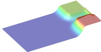
**Fig. 4.** Potential profile for  $Ta_2O_5$  water, salt, and biotin-streptavidin at  $\lambda = 10$  nm average distance. Blue denotes  $-1$  V while red stands for  $1$  V.
