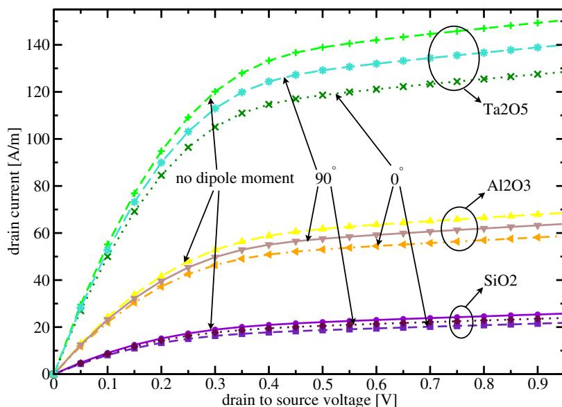
**Fig. 8.** Output curves for  $\text{SiO}_2$ ,  $\text{Al}_2\text{O}_3$ , and  $\text{Ta}_2\text{O}_5$  for calculation without dipole moment, angle  $0^\circ$  (perpendicular to surface), and angle  $90^\circ$  (parallel to surface).
