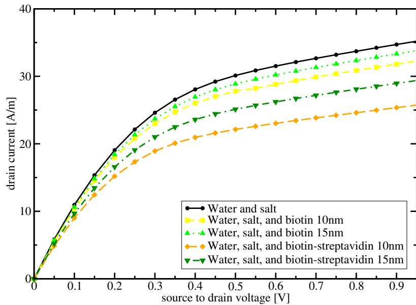
**Fig. 5.** Output curve for  $SiO_2$  for unprepared, prepared but unbound, and bound state at  $\lambda = 10$  nm and  $\lambda = 15$  nm, respectively.
