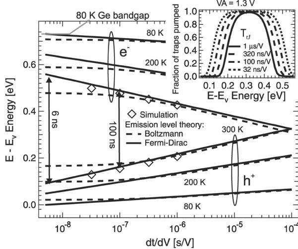
Fig. 2. Electron and hole emission levels calculated with Boltzmann [8] and Fermi-Dirac statistics as a function of pulse edge slew rate at different temperatures for germanium. (Inset) Simulation of the fraction of traps giving rise to CP current taking into account all emission and capture processes at 300-K. Equivalent emission levels from the simulation are compared with those from emission-level theory, showing the validity of the emission-level theory for germanium MOSFETs.
