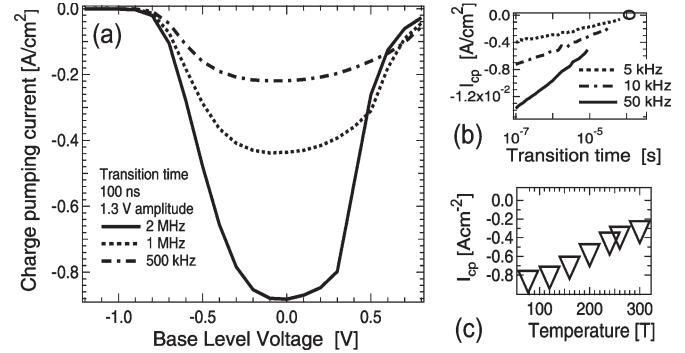
Fig. 3. (a) Ge MOSFET CP characteristics at 300-K show the typical hat shape and frequency scaling. (b) 300-K transition time sweep showing the point at which the CP current becomes zero. This corresponds to the time at which the hole and electron emission levels coincide. (c) CP current versus temperature increases in magnitude with decreasing temperature.
