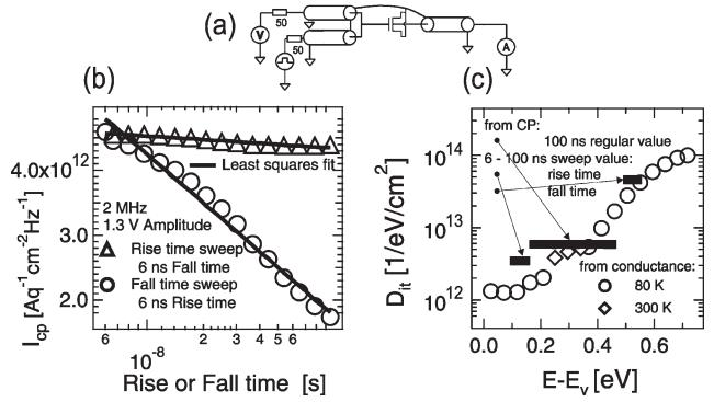
Fig. 1. (a) High-frequency setup used for CP with transition times down to 6 ns. (b) CP current as a function of rise and fall times down to 6 ns. The extracted characteristics using a least squares linear fit are shown in (c) as compared with an extraction using the full-conductance method.
