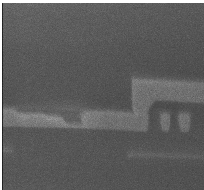
Fig. 7. FIB cross-section of interconnect after an electromigration test [13] (courtesy of Dr. Lucile Arnauld).
