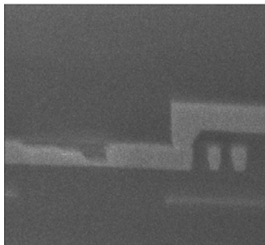
Fig. 7. FIB cross-section of an interconnect after an electromigration test [10] (courtesy of Dr. Lucile Arnaud).
