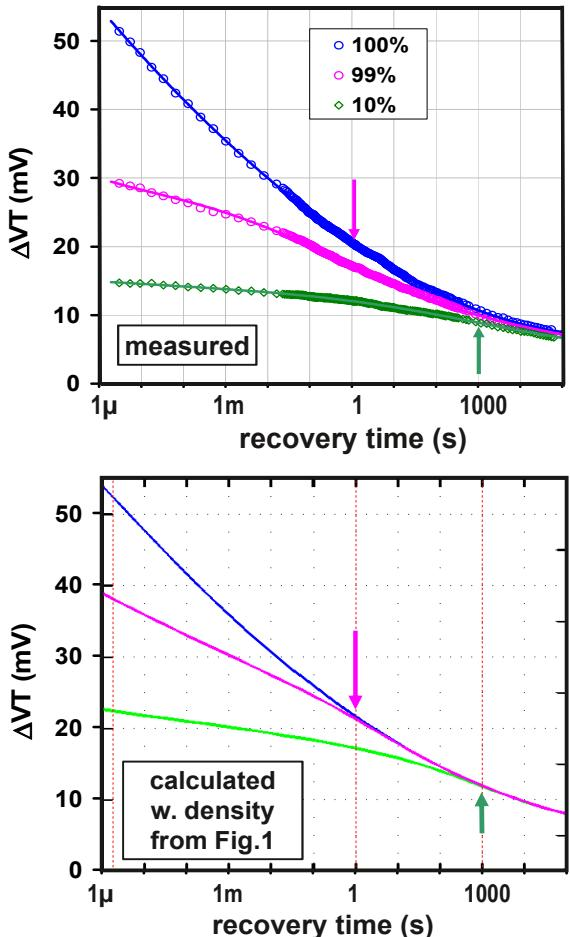
Figure 9 Measured and calculated recovery after stress with duty cycle 100% / 99% / 10%. The corresponding stress times  $t_{ac}$  were 100s/101s/1000s so that the net stress times  $t_{ac} \times \beta$  are the same for all 3 curves. Arrows mark the points where the AC recovery curves are supposed to merge with the DC curve (cmp. green arrows Fig. 4).
