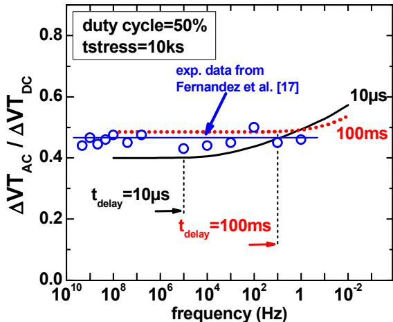
Figure 5: Frequency dependence, calculated with the model parameters from Fig. 1b in comparison with experimental data from ref.[17]. The experimental data were taken with a measuring delay  $t_D = 10$  s; the calculations have been done with  $t_D = 10$  us and 100 ms (see right hand labels). The frequency dependence vanishes for frequencies  $f > 1/t_D$ .
