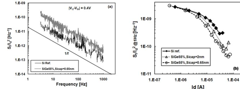
**Fig. 10:** (a) SiGe devices with a thin Si cap with optimized NBTI reliability show also reduced 1/f noise w.r.t. a Si ref. device with similar gate-stack, (b) and also w.r.t. a SiGe device with thicker Si cap.
