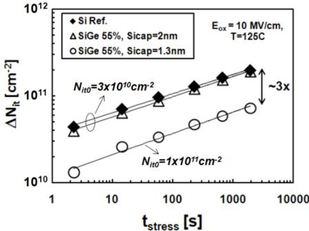
**Fig. 7:**  $\Delta N_{it}$  measured with charge pumping during NBTI stress at fixed stress conditions on a Si Ref. and on SiGe devices with a thick (2nm) and a thinner (1.3nm) Si cap.  $\Delta N_{it}$  follows a power law on the stress time with the same exponent ( $\sim 0.25$ ) on all three samples.
