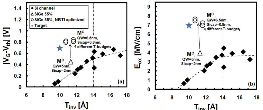
Fig. 5: A high Ge fraction (55%) and thick SiGe QW (6.5nm) combined with the use of a thin Si cap (0.8nm) boost NBTI lifetime to meet the target condition ( $|V_G - V_{th}|=0.7V$  at  $T_{inv}=10\text{\AA}$ , EOT~6\text{\AA}) on devices implementing aggressive IL scavenging ( $M^C$ ).
