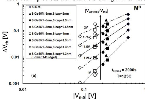
**Fig. 12:** (a, left) A clear correlation between the initial  $V_{th0}$  and  $\Delta V_{th}$  during NBTI stress was consistently observed on our SiGe devices with different gate-stacks: devices with lower initial  $V_{th0}$  always showed reduced  $V_{th}$  instability, at any given stress condition ( $|V_{Gstress} - V_{th0}|$ ). (b, right) This remarkable trend can be explained with the model proposed in Fig. 11.
