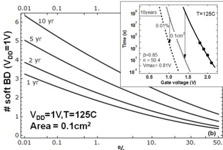
Fig. 6: Hot Carrier Injection (a) and Time Dependent Dielectric Breakdown (b) do not constitute a showstopper for our optimized SiGe device. In particular, < 6 soft breakdowns per chip (Area=0.1cm<sup>2</sup>) can be expected during application lifetime at  $V_{dd}=1V$  (inset documents extrapolation of TDDB data).
