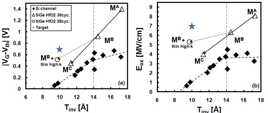
Fig. 3: (a)  $T_{inv}$  reduction by IL scavenging degrades the NBTI reliability faster than high-k scaling. (b) Converting operating gate overdrive to maximum operating  $E_{ox}$  shows that IL scavenging reduces SiGe maximum operating  $E_{ox}$  with the same slope observed for ultra-thin EOT Si devices implementing similar IL scavenging techniques.
