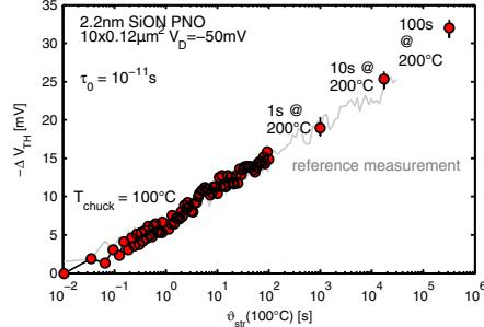
Fig. 13. Switching the device temperature to a higher value during stress accelerates the degradation. For small temperature switches, the correct interpretation of the acceleration can be demonstrated by a comparison with long-term OTF data (reference measurement).
