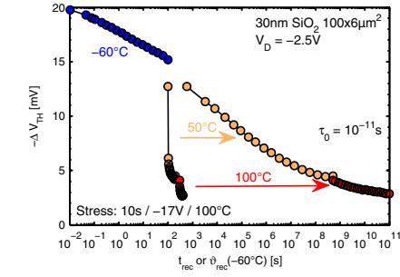
Fig. 5. When performing device temperature switches with the poly-heater during constant bias recovery at  $V_{TH}$ , substantial acceleration is observed [5]. Re-evaluation of the time data on the temperature-time scale results in a continuous recovery trace.
