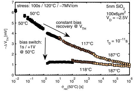
Fig. 6. Gate bias switches to positive values let defects with small time constants discharge quickly. The remaining degradation after the positive bias phase appears to be permanent but still undergoes slight recovery at long-enough times [10].
