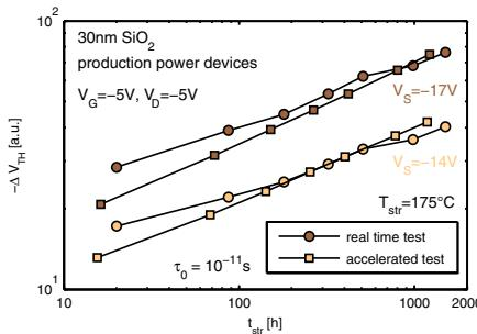
Fig. 16. Long-term NBTI degradation data of state-of-the-art power pMOS devices (gathered over several months) are reproduced within less than a day by using temperature accelerated testing with the poly-heater. Considering the vastly different measurement method used for the reference data, which included large (manual) delay times, which could only be roughly emulated by the poly-heater technique, the agreement is satisfactory.
