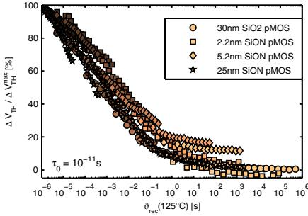
Fig. 4. The experiment of Fig. 3 was repeated on several different technologies with different gate dielectrics ( $\text{SiO}_2$  and PNO  $\text{SiON}$ ) and different gate oxide thicknesses. The temperature-time concept works for all observed technologies with one single value of  $\tau_0$ . The graph was normalized to the maximum drift 10ms post stress at  $-60^\circ\text{C}$ .
