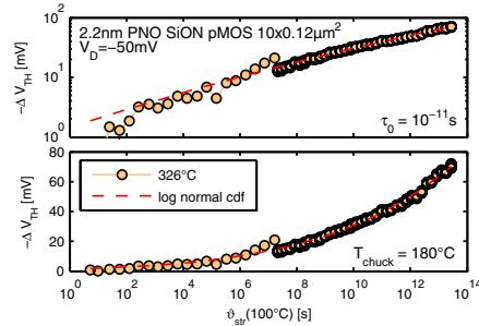
Fig. 14. Temperature accelerated OTF degradation data shows the same behavior as the data from interrupted stress measurements. Again, the saturation of the power law can be perfectly matched by a log-normal distribution of capture time constants.
