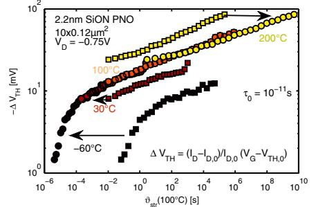
Fig. 15. Even without a poly-heater, the temperature-time concept is useful. The above shows OTF data measured at different chuck temperatures aligned onto a single degradation curve as a function of  $\vartheta$ . The only difference is that a correction for the degradation in  $I_{D,0}$  is needed. If  $I_{D,0}$  is performed with 10ms delay at 30°C one may add the drift after approximately 60s at -60°C to the 30°C data. With this approach all degradation traces can be aligned.
