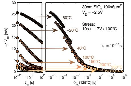
Fig. 3. On the left hand side recovery traces at different temperatures following exactly the same stress defined through temperature, duration and oxide field are depicted. On the right hand side the data was replotted as a function of the temperature-time. With a suitably chosen  $\tau_0$  all recovery traces can be matched.
