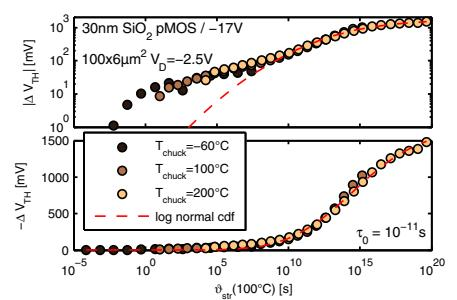
Fig. 12. In Fig. 11 we accelerated the test using one temperature and increasing stress times. Now, we always used 10s of stress but with increasing temperatures from  $T_{\text{chuck}}$  to the maximum achievable temperature with the poly-heater (upper plot of Fig. 8).
