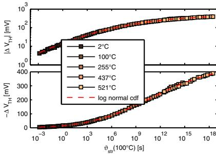
Fig. 10. When the data of Fig. 9 is corrected for the small offset due to the different active energy regions at different temperatures, it can perfectly be fitted by a log-normal cumulative distribution function (cdf) with large mean and large standard deviation.
