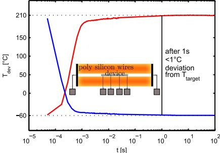
Fig. 1. The poly-heater consists of two poly-silicon wires situated next to the device. The electrical power supplied to the poly wires increases the device temperature and thus the drain current of the transistor. The rise of the drain current with turn-on of the heating power (red line) or turn-off (blue line) is converted to the change of the device temperature with time to reveal that the temperature settles close to its target value within less than a second [7].
