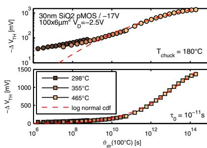
Fig. 11. Temperature accelerated interrupted stress measurements may also be performed on devices having 30nm  $\text{SiO}_2$  gate oxides. Again, long-term high-temperature data can be perfectly fitted by a log-normal distribution.
