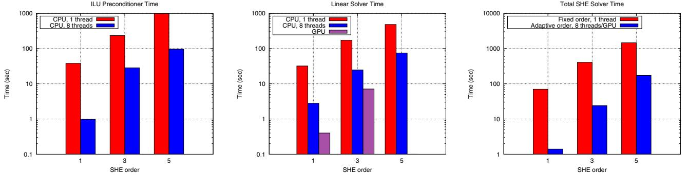
Figure 5: Comparison of execution times for the preconditioner setup (left), the linear solver run (center) and the gain of the complete SHE solver when using adaptive expansion orders. Benchmarks were carried out on a desktop machine equipped with a Intel Core i7 960 CPU, 12 GB RAM and a NVIDIA Geforce GTX 580 (out of RAM at order 5) on a coarse mesh in order to compare with high uniform expansion orders.
