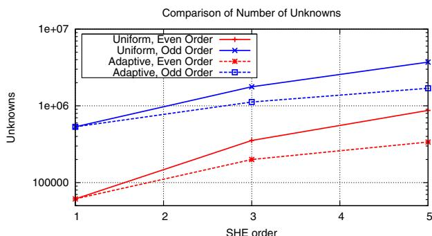
Figure 3: Comparison of the number of unknowns of the linear system on a coarse mesh in order to compare with high uniform expansion orders. The use of adaptive expansion orders leads to a reduction by a factor of more than two.
