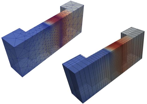
Figure 1: Comparison of the tetrahedral unstructured grid used for the simulation of a tri-gate transistor (no gate, oxide and body shown), and a structured grid with the same mesh size inside the channel. While the tetrahedral grid consists of 4838 points, the structured grid is made up of 27456 points, thus leading to considerably higher computational costs.
