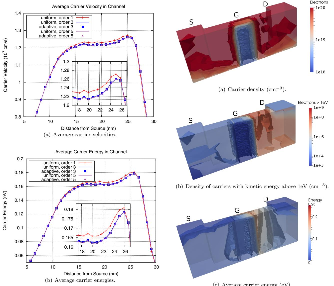
Figure 4: Average carrier velocities and energies for different uniform and adaptive SHE orders. Adaptive and uniform expansions yield identical results.
