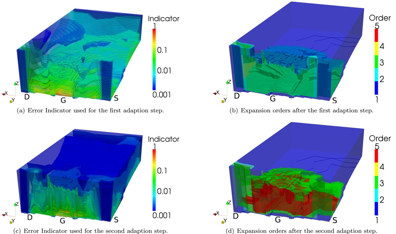
Figure 2: Based on the error indicator the expansion orders are locally increased. The bulk is kept at a fixed first order, since the contribution to transport is negligible. The z-axis denotes total energy.
