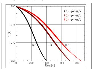
Fig.1. The time dependence of the sample temperature in response to periodic oscillations of the applied electric and magnetic fields with a relative phase shift of (a)  $\phi = -\pi/2$ , (b)  $\phi = -\pi/6$  and (c)  $\phi = -\pi/8$ .
