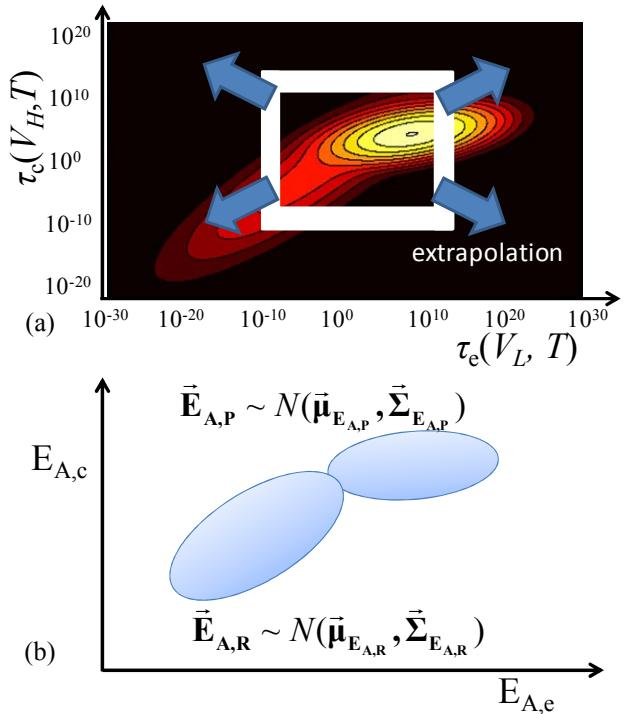
Figure 2. (a) Analytical fitting of the CET data to a bimodal bivariate log-normal distribution, (describing the “permanent” and “recoverable” BTI components) corresponds to (b) fitting the effective activation energy data to a bimodal bivariate normal distribution using Eq. 1. [8]
