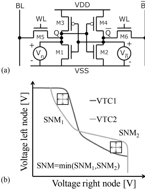
Figure 6. (a) The 6T-SRAM cell used for demonstration. (b) SNM margins are obtained by analyzing the butterfly curve during read mode, where the word and bit lines are set at the  $V_{DD}$  which is scaled according to the technology node used.
