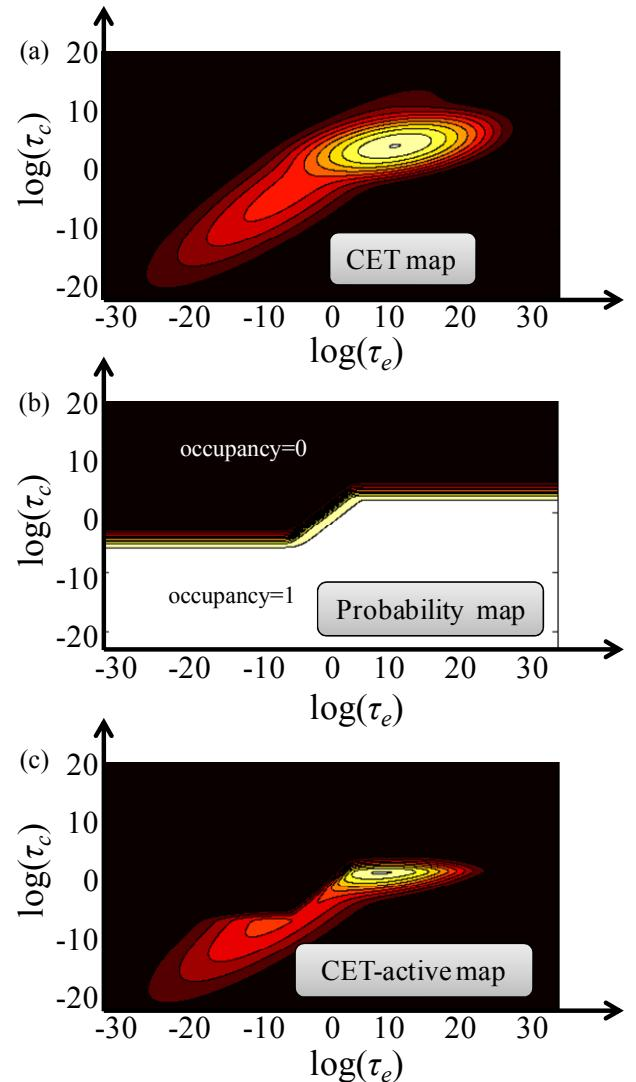
Figure 4. (a) The 2-component CET map, fitted on experimentally extracted data from large devices on the corresponding technology. (b) Occupancy probability map after an AC stress as function of  $\tau_e$  and  $\tau_c$  [12,13]. (c) The CET-active map is created by multiplying the occupancy probability map with the analytical CET map.
