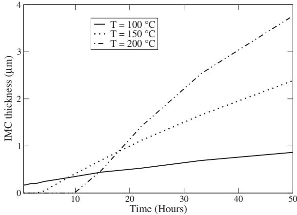
Fig. 7. Growth of IMC thickness in time. Fast migration of Cu and Ni at 150°C and 200°C prevents IMC emergence for several hours of stressing.
