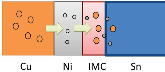
Fig. 2. EM of Cu and Ni atoms into Sn bump and the forming of IMC.
