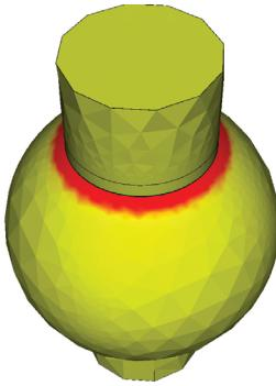
Fig. 5. IMC layer formed at the interface between a nickel UBM and a Sn solder bump.
