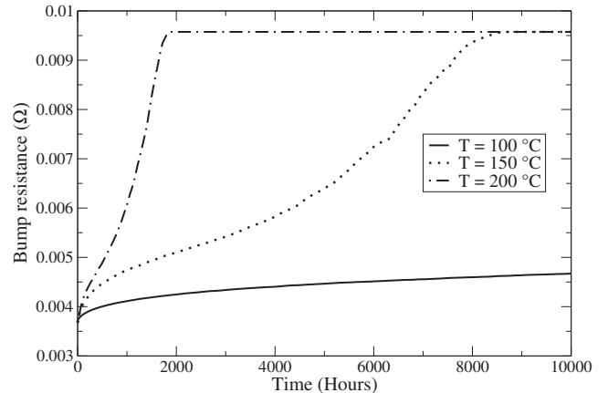
Fig. 8. Late phase of the resistance growth. The resistance of the solder bump increases, until the whole Sn is converted into IMC.
