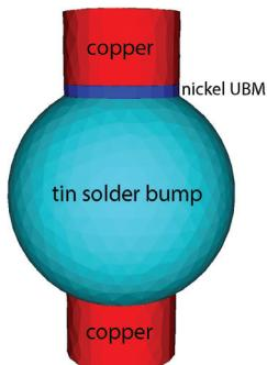
Fig. 4. Structure of the solder bump used for the study. On the top of the Sn bump a Ni UBM is placed.
