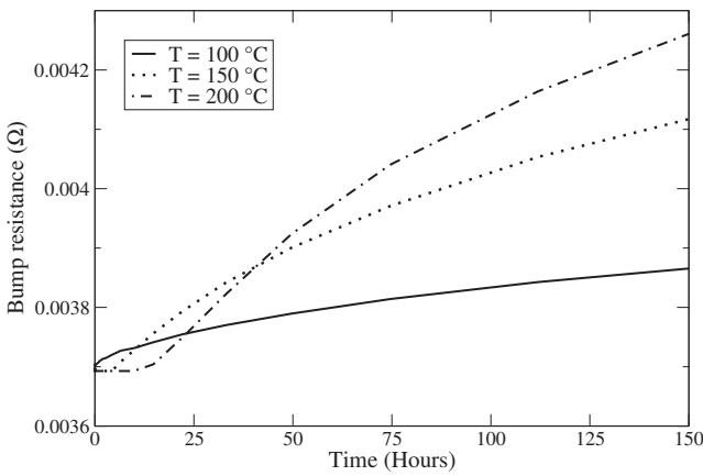
Fig. 6. Initial phase of solder bump resistance growth for three different temperatures.
