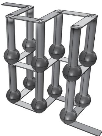
Fig. 3. Multilevel interconnect for 3D integration. Wafers are removed from the picture. Lighter color represents areas with higher current density. The copper TSV length is 100 μm and the diameter chosen 25 μm. The UBM thickness is 2.5 μm and the bump diameter is 40 μm. Due to the chosen geometry the lowest calculated current density is inside the bumps ( $2.66 \times 10^3 \text{ A/cm}^2$ ).
