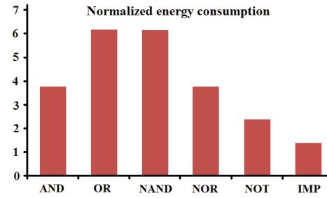
Fig. 4. The normalized energy consumption of IMP-based implementations of basic Boolean logic operations. The energy is normalized in the amount of that required for antiparallel-to-parallel MTJ switching ( $E_{AP \rightarrow P}$ ).
