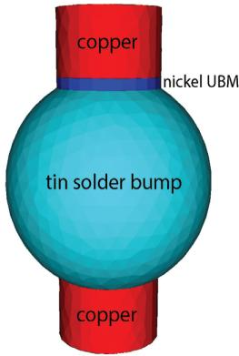
Fig. 5. Structure of the solder bump used for the study. On the top of the Sn bump a Ni UBM is placed.
