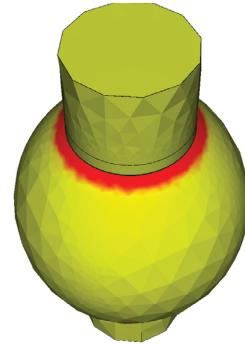
Fig. 6. IMC layer formed at the interface between a nickel UBM and a Sn solder bump.
