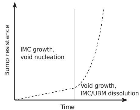
Fig. 2. Resistance change due to IMC growth and voiding with two different slopes.
