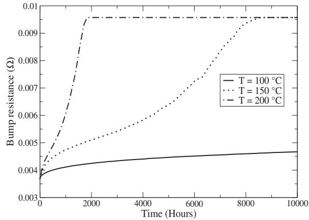
Fig. 9. Late phase of the resistance growth. The resistance of the solder bump increases, until the whole Sn is converted into IMC.
