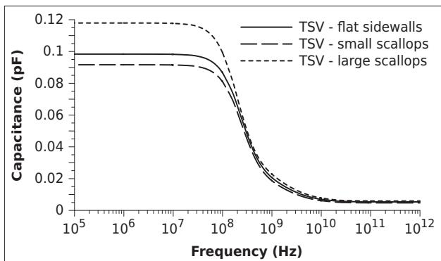
Fig. 5. Frequency-dependent capacitance (pF) for the three filled copper TSVs shown in Fig. 1.
