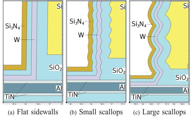
Fig. 3. Bottom of the three open tungsten TSVs with materials labeled. A variation in sidewall scallop height and width is evident.
