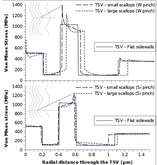
Fig. 12. Von Mises stress through the vertical middle of the open tungsten TSVs assuming a drop from a stress-free temperature of  $320^\circ\text{C}$  to  $20^\circ\text{C}$ .
