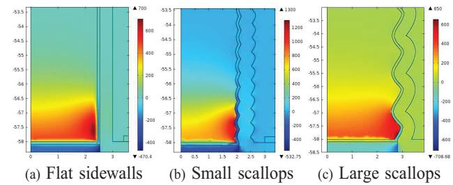
Fig. 8. Electromigration-induced stress (MPa) accumulation at the bottom of the three filled copper TSVs when a 1A current is applied through the top of the structure for 700hrs.
