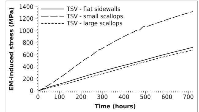
Fig. 9. Maximum EM-induced stress (MPa) through the filled copper TSVs during operation at a 1A current.
