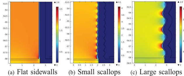
Fig. 7. Current density distribution ( $\text{MA}/\text{cm}^2$ ) in the three filled copper TSVs when a 1A current is applied through the top of the structure.
