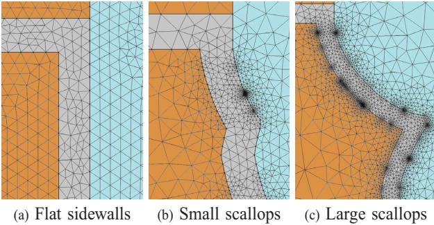
Fig. 2. Mesh at the top of the three filled copper TSVs. The image is an enhanced section from Fig. 1 where the oxide, copper, and tantalum layers are visible.
