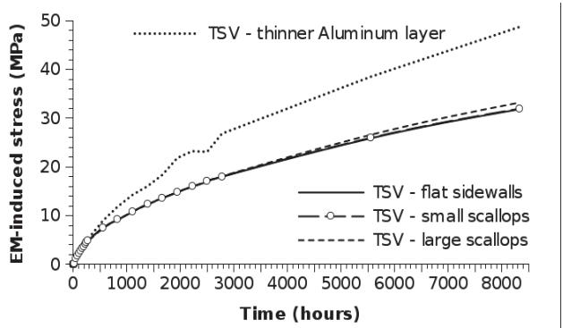
Fig. 15. Maximum EM-induced stress (MPa) through the aluminum layer in the open tungsten TSVs, while operating with a 1A current applied through the structure.
