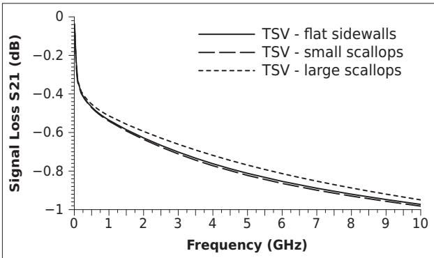
Fig. 11. Frequency dependence on the signal loss S21 (dB) for the three open tungsten TSVs. A higher loss is noted at high frequencies for the large-scalloped structure.
