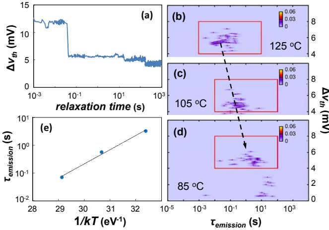
Fig. 9: (a) Illustration of a single relaxation transient of a single small nFET. (b-d) TDDS: A selected single electron trap emission (note the “shifting” with  $T$  of defect cluster due to multiple perturbations/ transients) is strongly thermally activated,  $E_a = 1.18$  eV in this particular case (e) [12].
