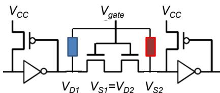
Fig. 12: Node and additional breakdown leakage path definitions used in our SPICE simulations.
