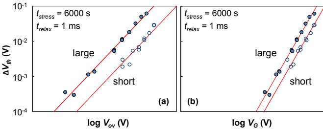
Fig. 8: (a) Voltage overdrive  $V_{ov}$  and (b) gate voltage  $V_G$  acceleration of PBTI degradation of large and short devices. Short devices degrade less, likely due to thicker gate oxide.
