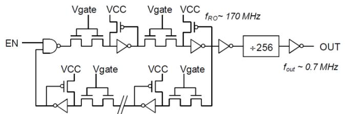
Fig. 2: The ring oscillator (RO) test circuit consists of 127 stages and oscillates at  $\sim 170$  MHz at operating conditions [6]. Serially connected nFETs are placed between each RO stage and are controlled by a separate terminal  $V_{gate}$ . The rest of the circuit is using supply voltage  $V_{CC}$ .
