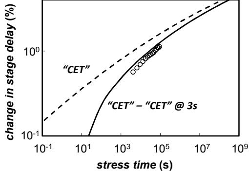
Fig. 3: Change in RO frequency (symbols, normalized to the first reading in 3 s), converted into change in delay per stage, measured at stress  $V_{gate}$ , is excellently matched by the projection based on the PBTI CET map (lines).
