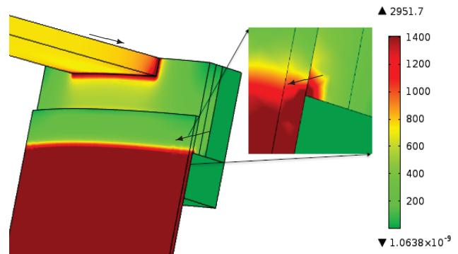
Fig. 3. Current density in the structure ( $\text{A}/\text{cm}^2$ ). The inset is a zoom-in at the corner of the aluminium/tungsten interface.
