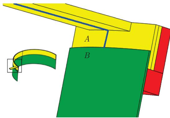
Fig. 2. TSV structure showing aluminium in yellow, tungsten in green, and silicon oxide in red. The blue line indicates a cut through the TSV for use in the subsequent figures.
