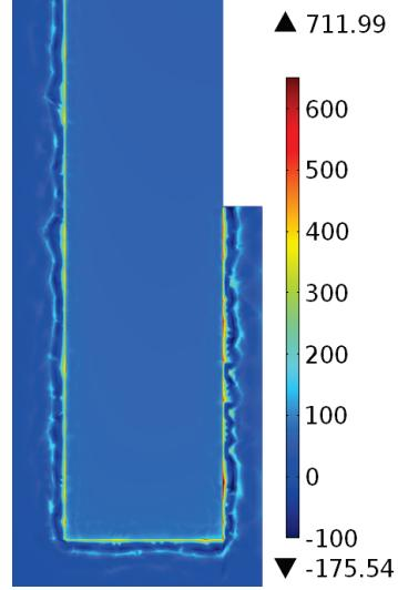
Fig. 7. Tensile stress (in MPa) after  $t=10^6$ s of current flow. A surface cut along the red line of Fig. 1 is shown. Red colour indicates the stress peak.
