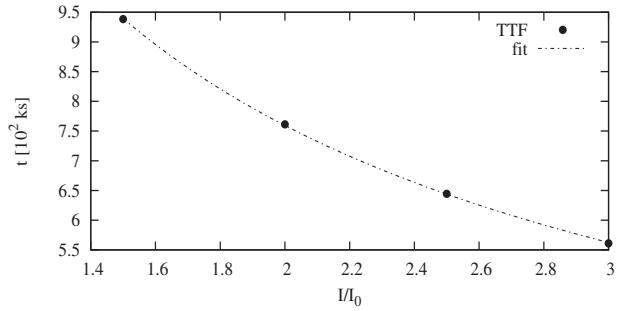
Fig. 11. Simulated TTF for different current densities. Broken line shows the exponential fitting of the results.
