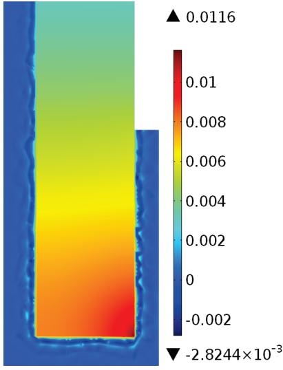
Fig. 4. Relative vacancy concentration change compared to the vacancy equilibrium concentration after  $t=1$ s of current flow. A surface cut along the red line of Fig. 1 is shown. Red colour indicates the peak concentration.
