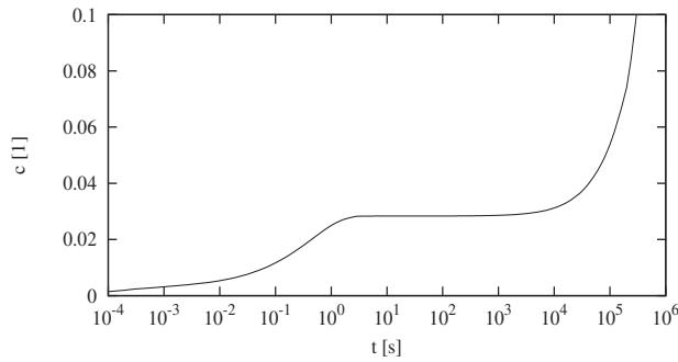
Fig. 9. Maximum relative vacancy density change versus time. Located at the aluminium/tungsten interface.
