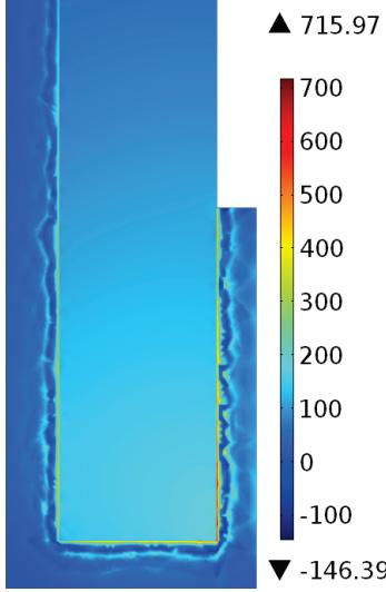
Fig. 5. Tensile stress (in Pa) after  $t=1$ s of current flow. A surface cut along the red line of Fig. 1 is shown. Red colour indicates the peak tensile stress.
