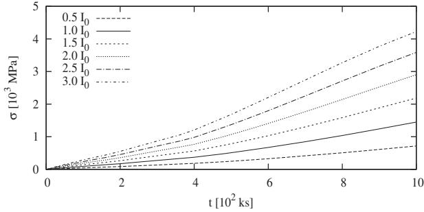
Fig. 10. Stress build up in the TSV for different current densities.  $I_0$  is the current used for Fig. 8 and Fig. 9.
