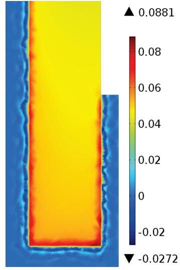
Fig. 6. Relative vacancy concentration change compared to the vacancy equilibrium concentration after  $t=10^6$ s of current flow. A surface cut along the red line of Fig. 1 is shown. Red colour indicates the peak concentration.
