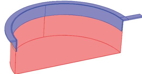
Fig. 1. TSV structure: Aluminium in blue and tungsten in red. The tungsten cylinder is shortened to 10% of the real length. For the simulated TSV the upper plate is removed.
