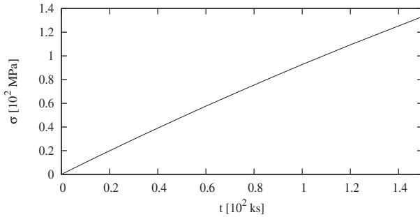
Fig. 8. Maximum stress versus time at the aluminium/tungsten interface.
