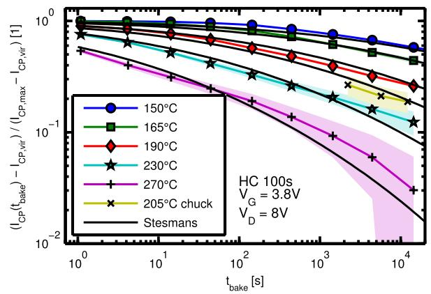
Fig. 3. Baking the device at zero gate and drain bias decreases the number of HC-induced traps visible in the maximum CP current. It is thereby insignificant whether the temperature is provided by the poly-heater (standard case in this letter) or the thermo chuck (trace labeled chuck). The shaded areas correspond to the confidence intervals of the  $I_{\text{CP}}$  measurement. In addition, the result of a fit to the model by Stesmans (1) [8] is shown.
