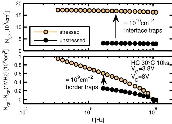
Fig. 1. Frequency-dependent CP measurement before and after HC stress. The HC stress increases the number of interface traps, here defined as traps with emission and capture time constants smaller than  $\approx 0.5 \mu\text{s}$  (upper plot). In contrast, the number of border traps (here defined as traps with time constants larger than  $\approx 0.5 \mu\text{s}$ ) created during HC stress is roughly one order of magnitude smaller.
