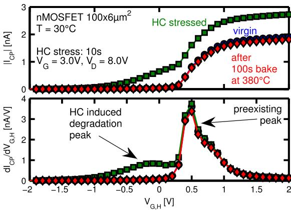
Fig. 2. Upper plot shows constant base level ( $-5 \text{ V}$ ) CP characteristics at  $625 \text{ kHz}$  with rising and falling slopes of  $50 \text{ nA/V}$ . The HC-induced increase in the CP current can be fully removed with the short bake phase. The derivative of the characteristics (bottom plot) shows that the increase of the  $I_{\text{CP}}$  is due to a second degradation-induced peak that is due to the strongly localized buildup of charges near the drain junction [10].
