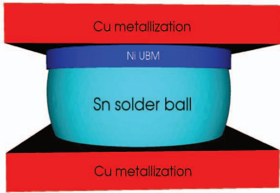
Fig. 1. Solder bump structure used for simulation.
