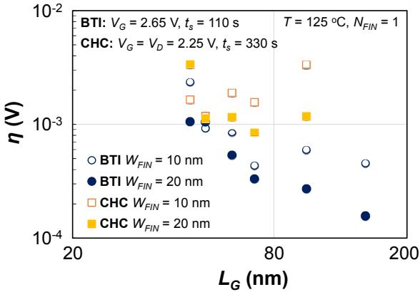
Fig. 8: Gate length dependence of BTI and CHC variability in long nFinFETs, as extracted from MPs (cf. Fig. 1). BTI  $\eta$  dependence follows  $A_G^{-1}$  scaling, while CHC  $\eta$  is higher, approx. constant and hence tends to converge at shorter gate lengths.
