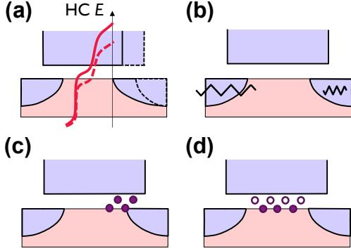
Fig. 4: Sources of increased CHC variability: (a) Channel length/LER and schematic CHC energy distribution, (b) series resistance, (c) longitudinally and (d) vertically non-uniform trapping.
