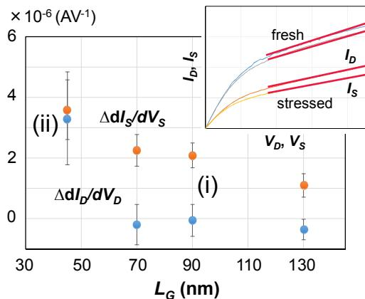
Fig. 9: Change in  $dI_d/dV_d$  ( $dI_s/dV_s$ ) slope after CHC stress (inset) allows visualizing CHC degradation (i) longitudinally localized in longer nFinFETs and (ii) spanning the entire channel in shorter devices. BTI degradation is symmetric at all  $L_G$ 's (not shown).
