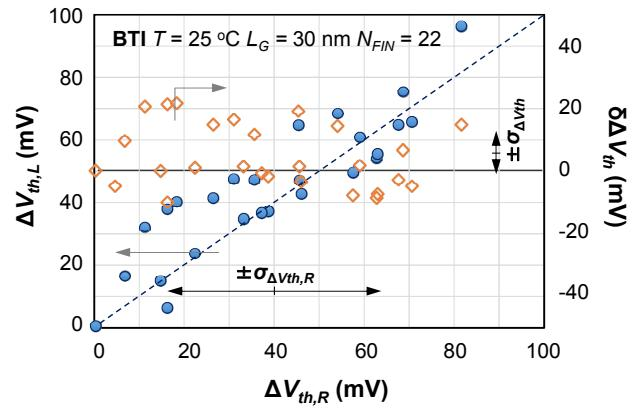
Fig. 2: Illustration of an extreme case of across-wafer variability affecting time-dependent variability due to BTI stress. Note the correlation  $\Delta V_{th,L}$  and  $\Delta V_{th,R}$  in individual MPs due to the systematic variability (solid circles) and the reduction of variance  $\sigma_{\Delta V_{th}}$  when Eq. 3 is used on the MP degradation difference  $\delta\Delta V_{th}$  (Eq. 2, open diamonds).
