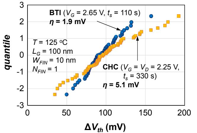
Fig. 3: For the same mean degradation, CHC stress in nFinFETs results in a wider distribution, as compared to uniform BTI stress.
