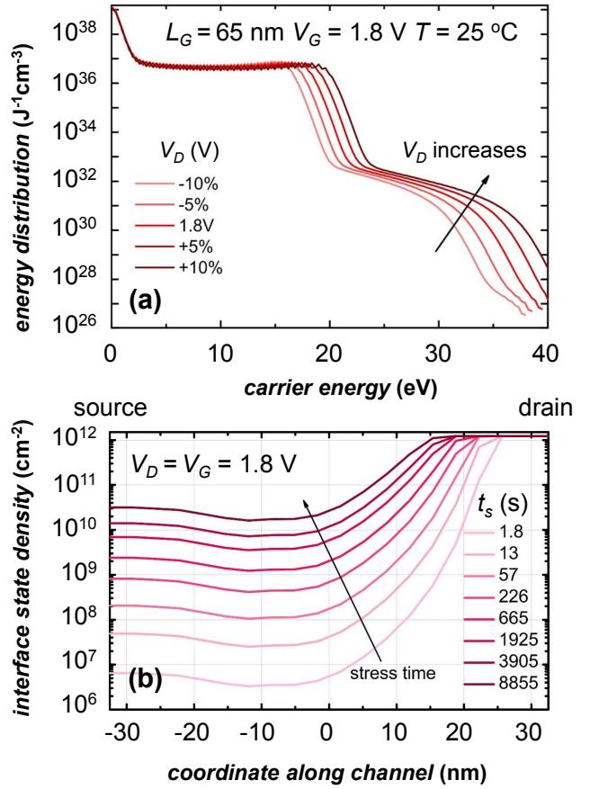
Fig. 6: CHC simulation in a planar device. (a) CHC energy distribution at drain (cf. Fig. 4a), responsible for trap generation and charging, is sensitive to drain bias. (b) Increase in CHC degradation along the channel. Note the most damaged region extending ~20 nm from the drain.
