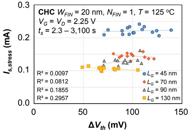
Fig. 7: Channel current during stress is not correlated with degradation (result for  $W_{FIN} = 20$  nm shown), disqualifying series resistance as a main source of increased CHC variability. Stress time  $t_s$  is adjusted per  $L_G$ .
