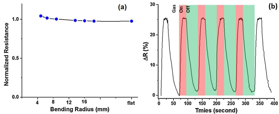
**Fig. 6.** (a) normalized resistance of the Cu-SWCNTs-based flexible devices as a function of the bending radius and (b) the sensor response upon exposure to 20 ppm  $\text{H}_2\text{S}$  gas and a bending radius of 7.8 mm.
