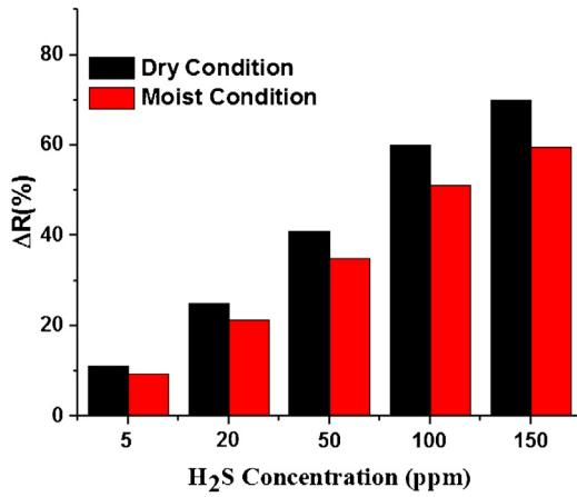
**Fig. 7.** Final response of the Cu-SWCNTs based flexible sensor under 40% relative humidity and dry environment at room temperature.
