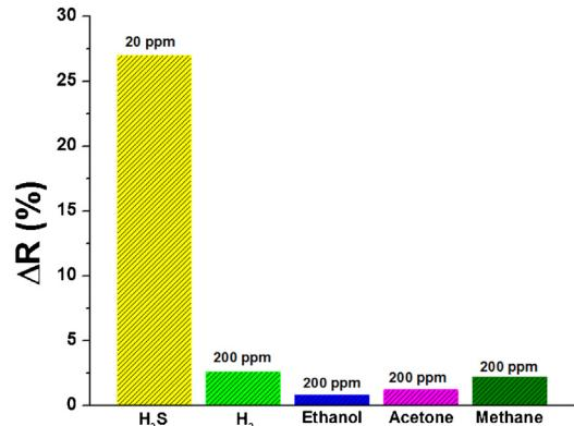
**Fig. 5.** The selectivity of the fabricated sensors to various gases. The H<sub>2</sub>S concentration is kept at 20 ppm while the concentrations of other interfering gases are fixed at 200 ppm.
