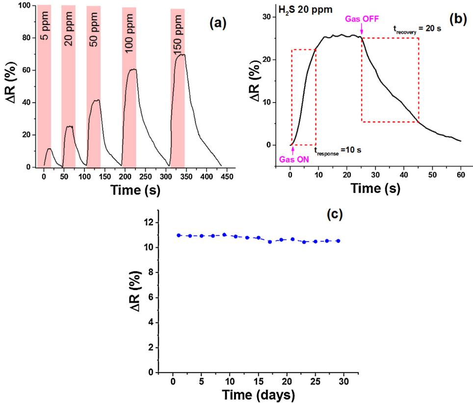
**Fig. 4.** (a) Sensor response to various H<sub>2</sub>S gas concentrations at room temperature. (b) Enlarged response curve of the sensor under exposing to 20 ppm H<sub>2</sub>S (c) Long-term evaluation of the sensor's response to 5 ppm H<sub>2</sub>S gas at room temperature.
