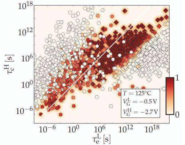
Fig. 7: Based on  $\tau_c(V_G)$  and  $\tau_e(V_G)$  dependences (cf. Fig. 6) of a population of defects, a CET map can be computed [19,20].  $\tau_c^H = \tau_c(V_G^H)$  and  $\tau_e^L = \tau_e(V_G^L)$  define where a defect contributes in the CET map and the average contribution of a defect to  $V_{th}$  (0-1 gradient scale) is given by its equilibrium occupancy difference and its distance from the substrate [20].
