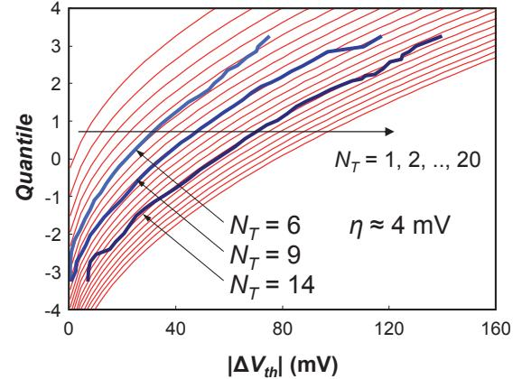
Fig. 11: Total  $\Delta V_{th}$  distribution (Eq. 2) for the average number of defects  $N_T$  from 1 to 20 (thin lines) rescaled to fit experimental distributions from Fig. 10 of Ref. [34], with the corresponding values of  $N_T$  and  $\eta$  readily extracted.
