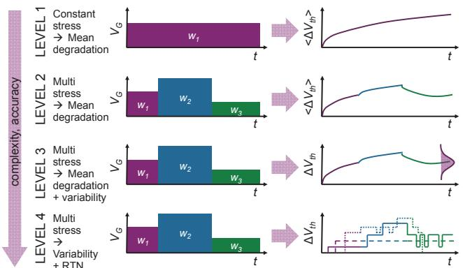
Fig. 14. Complexity/accuracy levels of incorporating device aging (specifically here, the threshold voltage shift) in circuit simulations. The full workload on each device can be *approximated* by a series of phases  $w_i$  with duration  $t$ , voltage  $V$ , duty factor  $DF$ , frequency  $f$ , and temperature  $T$ . (In reality the number of workload phases is typically very large.)
