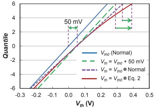
Fig. 13: Three ways of adding time-dependent variability to time-zero distribution (solid straight line): i) a simple shift of  $\langle \Delta V_{th}(t) \rangle$  in all devices (dashed line), ii) a Normal (Gaussian, dotted line), and iii) the defect-centric statistics given by Eq. 2 (solid curve). Discrepancies with respect to the defect-centric model at  $6\sigma$  are demarcated [36].
