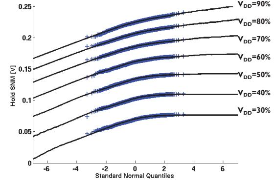
Fig. 16: Hold SNM distribution at decreasing supply voltage  $V_{DD}$ . Lines: the non-MC numerical propagation technique can predict the tails of the distribution up to  $\pm 7\sigma$ . Symbols: MC simulation added for comparison shows excellent agreement with the non-MC method [51].
