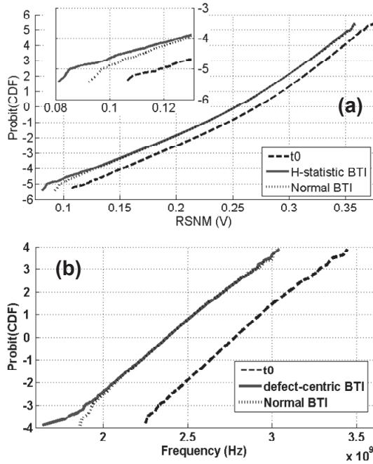
Fig. 15: (a) Probit plot of the Read Signal Noise Margin (RSNM) of 28nm technology SRAM cell for an average 50mV NBTI shift. (b) Impact of binning at time-zero. Using the yield criterion of *mean*- $\sigma$  on the ring oscillator frequency distributions results in a wider discrepancy between the defect-centric and Normal degradation statistics [49].
