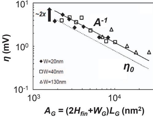
Fig. 9: The average impact per trap  $\eta$  as  $A_G^{-1}$  in pFinFETs (high-k/MG,  $t_{inv} \approx 1.7\text{nm}$ ) with varying fin width  $W_G$  and gate length  $L_G$  (fin height  $H_{fin}$  is fixed). Each point is extracted from a distribution such as those in Fig. 8. The value of  $\eta$  is  $\sim 2\times$  higher than the expected  $\Delta V_{th}$  for a single charge from a charge sheet approximation  $\eta_0 = q/C_{ox}$  [29].
