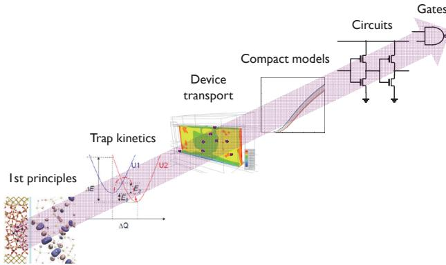
Fig. 3: Hierarchical levels of the defect-centric picture: Understanding of defect properties at the atomic level [6] can be propagated up to circuit design.
