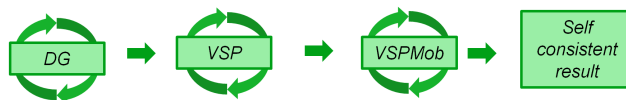
Figure 3. The iteration scheme for device simulation with self-consistent quantum correction and mobility evaluation comprises three blocks: block I - empirical models for density and mobility are run; block II - self-consistent quantum correction provided by VSP is used with empirical mobility models; block III - self-consistent quantum correction and mobility provided by VSP are used. Each block is iterated until convergence is achieved.
