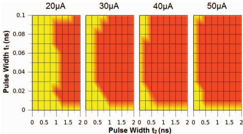
Figure 6. Schematic illustration of the dependence of the switching probability for the “two write pulses” scheme on the current and pulses width. The dependences are shown for four current values: 20 $\mu$ A, 30 $\mu$ A, 40 $\mu$ A, and 50 $\mu$ A. For switching probability estimation, 100 simulations of switching were performed on each combination of pulses’ widths.
