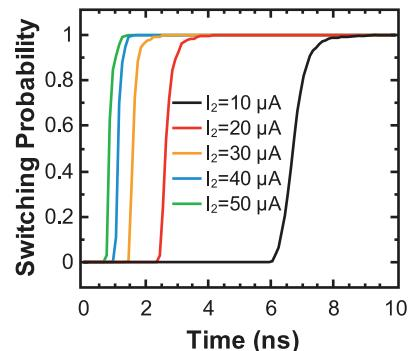
Figure 5. Switching probability for the "write pulse 2" scheme as a function of the pulse duration for five current values. For switching probability estimation, 250 simulations of switching were performed on each current value.
