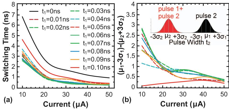
Figure 8. (a) Switching time as a function of current. (b) The difference between the minimum value of the pulse width  $t_2$  required to achieve a non-zero probability of switching by using the "write pulse 2" scheme ( $\mu_1-3\sigma_1$ ) and a value of the pulse width  $t_2$  needed to achieve guaranteed switching with the "two write pulses" scheme ( $\mu_2+3\sigma_2$ ) as a function of current.
