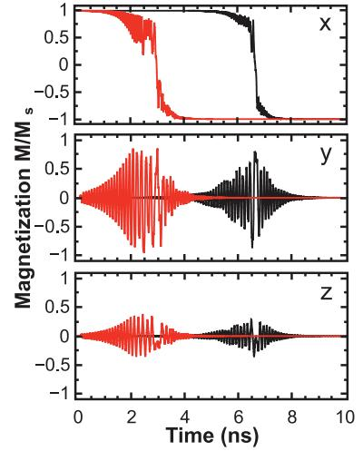
Figure 3. Magnetization components as a function of time: (top)  $x$ -component; (middle)  $y$ -component; (bottom)  $z$ -component. The current is  $10 \mu\text{A}$ . The "two write pulses" scheme is shown in red and the single "write pulse 2" scheme is shown in black.
