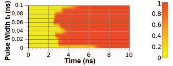
Figure 4. Switching probability for the "two write pulses" scheme as a function of the time for different values of pulse width  $t_1$ . For switching probability estimation, 250 simulations of switching were performed on each pulse width  $t_1$ .
