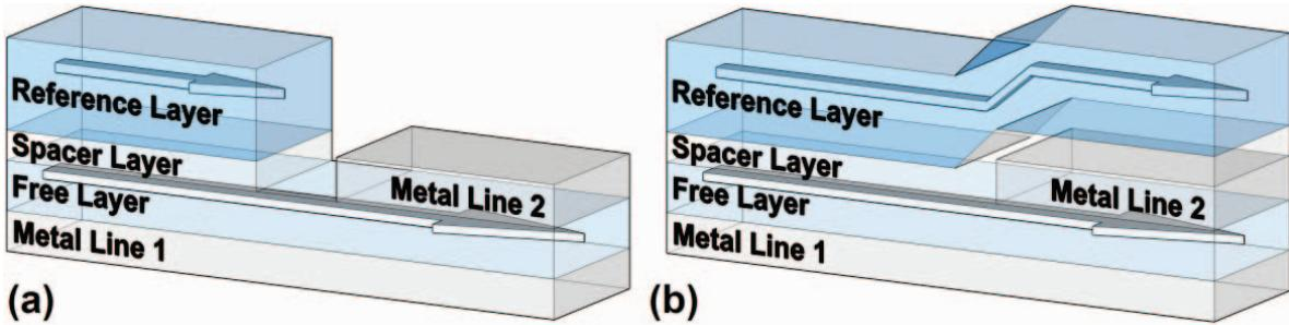
Figure 9. Schematic illustration of two memory cell structures with switching of the free layer based on the proposed "two write pulses" scheme.
