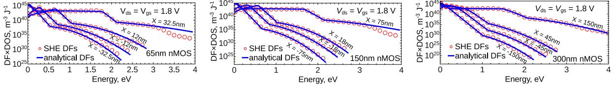
**Fig. 2.** The electron DFs simulated with ViennaSHE and with the DD-based model for three nMOSFETs with gate lengths of 65, 150, and 300 nm for  $V_{\text{gs}} = V_{\text{ds}} = 1.8$  V plotted at different positions in the device. The source is at  $x = -L_{\text{G}/2}$  and the drain is at  $x = C L_{\text{G}/2}$ . The DFs are obtained for 25 °C.
