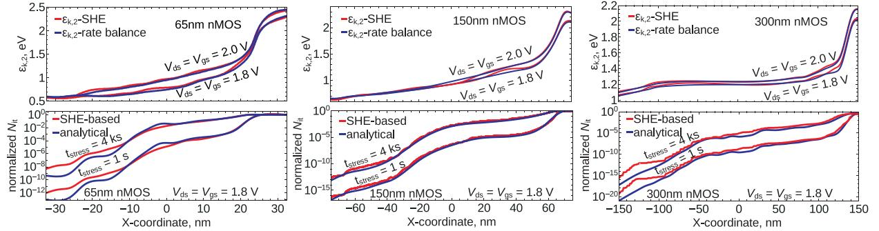
**Fig. 3.** Upper panels: The knee energy  $\epsilon_{k,2}$  ( $x$ ) for all three devices obtained for the same stress conditions as in Fig. 2. Lower panels: The normalized (to the concentration of Si-H bonds)  $N_{it}$  ( $x$ ) profiles, evaluated using DFs obtained with our analytic model and with ViennaSHE. Results are for  $T = 25^\circ\text{C}$ .
