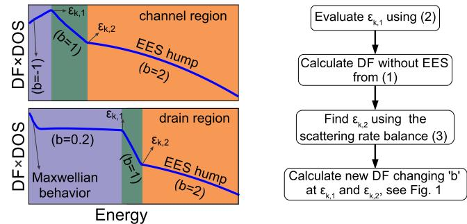
**Fig. 1.** Left panel: A schematic representation of the carrier DFs for the channel region (upper panel) and the drain region (lower panel) with the values of parameter  $b$ . Right panel: flowchart for the calculation of the carrier DF.
