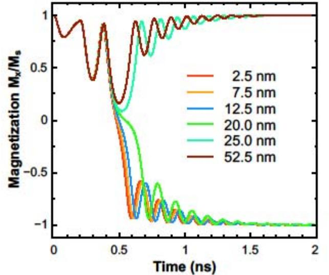
Fig. 4. The magnetization dynamics for several overlap lengths of wire NM2. Two consecutive perpendicular pulses with 30μA current and 200ps duration are applied.
