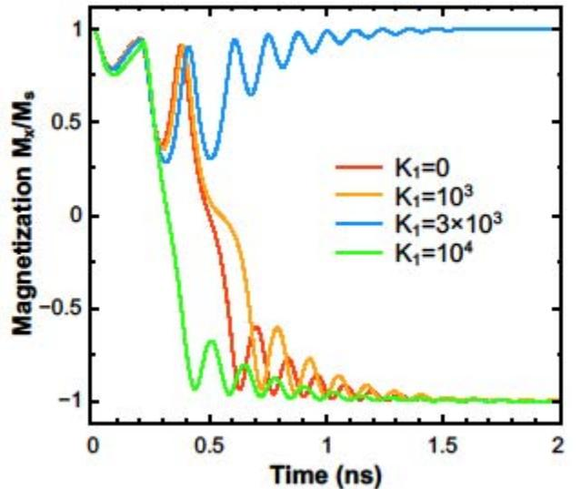
Fig. 6. Adding perpendicular magnetization if a two-pulse scheme allows to reduce the current by a factor of 6 for sub-0.5ns switching.
