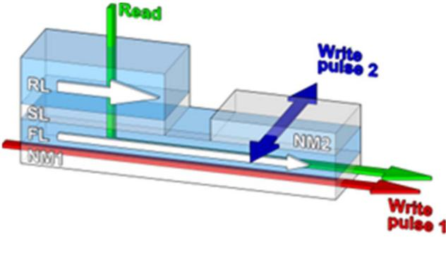
Fig. 1. Schematic of the in-plane SOT-MRAM cell. The free layer of an MTJ is grown above the heavy metal wire NM1, through which the current pulse is applied. The wire NM2 serves to conduct the perpendicular current “Write pulse 2” of the in-plane SOT-MRAM cell.
