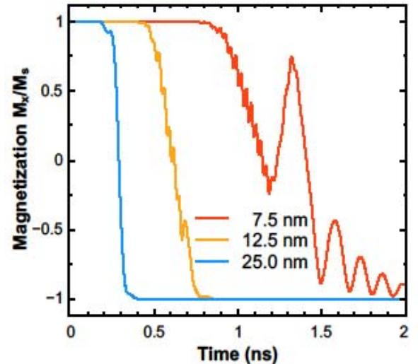
Fig. 2. Time dependent magnetization evolution for several values of the second wire NM2 overlap. The current is scaled with NM2 and is equal to  $180\mu\text{A}$  for  $\text{NM2}=25\text{nm}$ ,  $90\mu\text{A}$  for  $\text{NM2}=12.5\text{nm}$ , and  $54\mu\text{A}$  for  $\text{NM2}=7.5\text{nm}$ .
