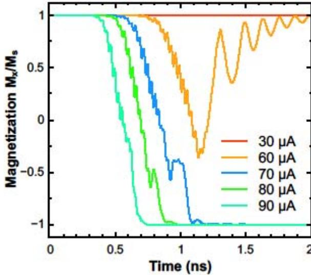
Fig. 3. Time evolution of the magnetization for several values of the current through wire NM2 with the width 12.5nm. The current through wire NM1 is zero.
