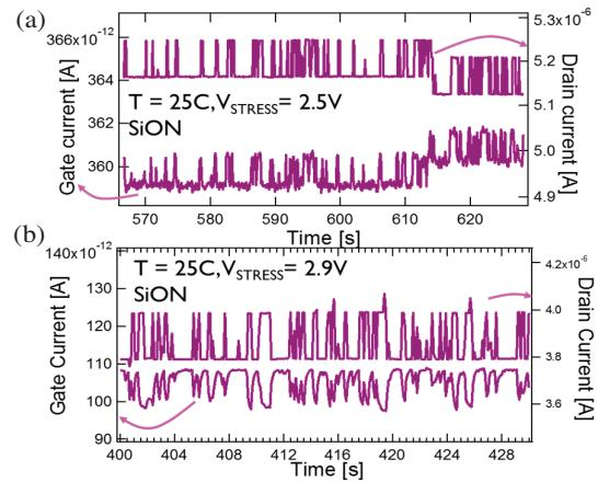
Fig 9 Both (a) positive and (b) negative  $I_G/I_D$  correlations are measured on separate SiON nFETs after stress. The negative correlation in (b) also shows signs of a second RTN path in the drain current, and is superimposed both on the low and the high state of the signal, but not visible in the gate current.
