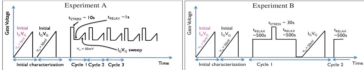
Fig. 3. Schematic illustration of the experiments performed. Experiment A provides learning about the *stress dependent evolution* of the SILC as it is focused on measuring  $I_GV_{GS}$ s after intermittent stress cycles. The cycles are repeated 100 times. Experiment B focusses on the *time evolution and correlation* of both the gate and drain current after one short stress phase. During  $t_{RELAX}$  correlations between RTN in  $I_G$  and  $I_D$  are measured, as well as  $I_B$ .
