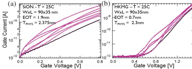
Fig. 4. Initial  $I_DV_G$ s for different (a) SiON and (b) HKMG devices with similar physical thickness. In both cases, only a few devices show a near-perfect exponential leakage current (black lines). Other devices show an inflected  $I_DV_G$ , indicating the presence of at least one TAT-leakage path.
