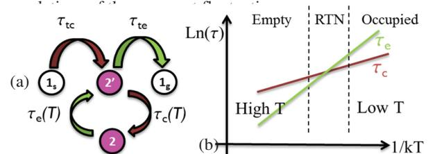
Fig 2. (a) The trap-assisted tunneling model as proposed by [9] and [10], and (b) typical temperature dependence of the time constants characterizing the transition between metastable states 2' and 2.
