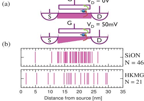
Fig. 5. (a) The linear drop over the channel potential allows to extract the lateral position of the TAT-paths, using the  $V_D$  dependence of the  $I_{G\_TAT}$  curves. (b) The SiON traces show a more centered distribution of TAT-paths than the HKMG devices.
