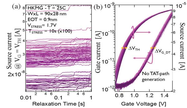
Fig. 6. (a) Experiment A performed on a HKMG device (WxL: 90x28nm, EOT = 0.9nm) for one stress voltage. Relaxation traces of the device after subsequent stresses shows tens of charges being trapped. (b) The  $I_DV_G$  and  $I_GV_G$  traces after the short relaxation show a comparable total  $V_{TH}$  shift for both drain and gate currents, but no TAT-paths have been created.
