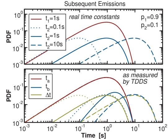
Fig. 5: Scenarios B/C: **Top:** As in Fig. 4, but now for two defects subsequently emitting a hole. **Bottom:** The distribution of the first emission event  $t_a$  recorded by TDDS is of course identical to that of  $t_1$ , while the distribution  $t_b$  is narrower than exponential. Most importantly, however, the distribution of  $\Delta t$  can clearly reveal the case where the second emission event quickly follows the first.
