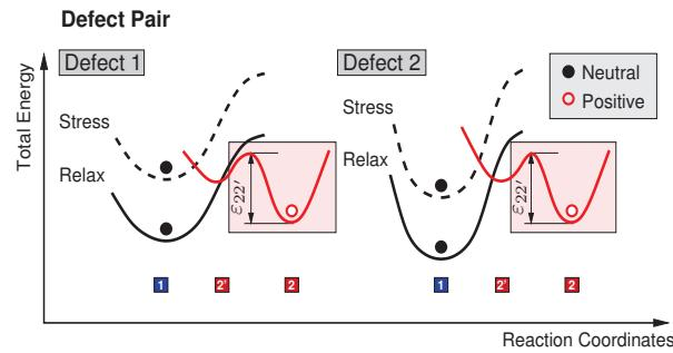
Fig. 12: For two independent defects to incidentally have similar emission time constants, the thermal barriers connecting states 2 and 2',  $\varepsilon_{22'}$ , must be similar. The circumstances for this to happen remain to be clarified.
