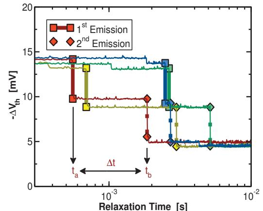
Fig. 2: Typically, in each trace only a single emission event is observed per cluster. However, particularly for larger stress times, two emission events can sometimes be observed. Here, four example traces contributing to the 175 °C spectral maps of Fig. 1 are shown. The step-heights of the second emission event are within 5% of those of the first emission event. Note that the emission events  $t_a$  and  $t_b$  do not directly correspond to the emission times of the defects as discussed below.
