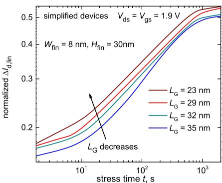
Figure 9:  $\Delta I_{d,lin}(t)$  traces simulated for three different series of devices: with varying  $L_G$ ,  $W_{fin}$ , and  $H_{fin}$  for  $V_{ds} = V_{gs} = 1.9$  V.
