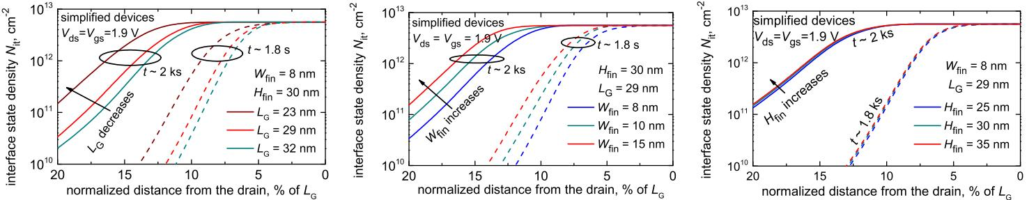
Figure 10: The  $N_{it}(x)$  profiles simulated for three series of simplified devices with varying  $L_G$ ,  $W_{fin}$ , and  $H_{fin}$  stressed under  $V_{ds} = V_{gs} = 1.9$  V; stress times are  $\sim 1.8$  s and  $\sim 2$  ks. They are shown along the top/sidewall edge of the fin and  $x$  axis represents the distance from the drain (in % of  $L_G$ ). One can see that the  $N_{it}$  front propagates deeper inside the fin at longer stress times and as the stress bias grows.
