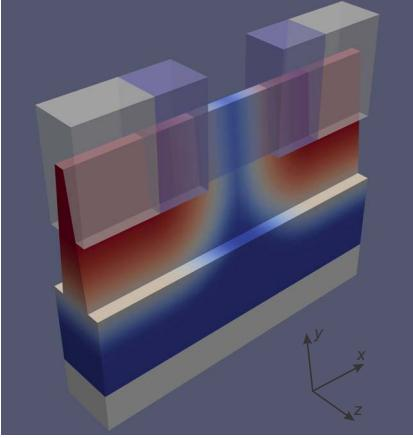
Figure 1: Schematic representation of the real FinFET used for HCD measurements and model verification.
