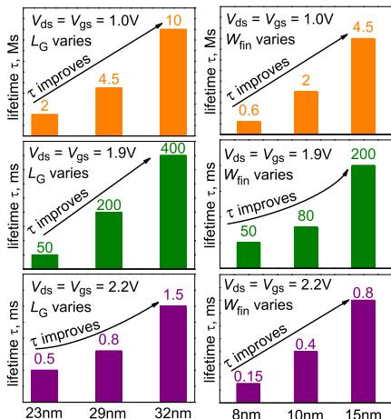
Figure 13: Summary of device lifetime values extracted for simplified FinFETs.
