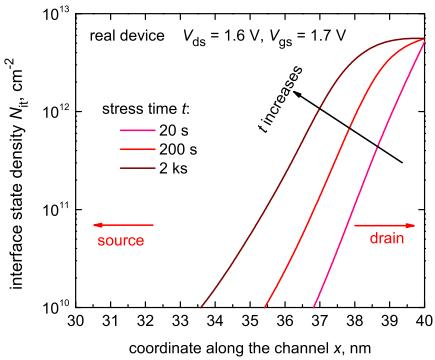
Figure 4: The evolution of the  $N_{it}$  density with stress time (left) and stress bias (right) for the real device. The  $N_{it}$  profile is shown for the same cut as DFs in Fig. 2. For the sake of visibility we show only the drain peak of  $N_{it}$  (the drain is at  $x = 40$  nm, source is at  $x = 0$ ).
