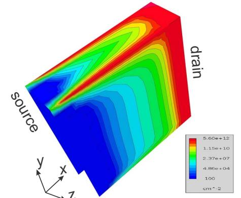
Figure 7: Electron DFs calculated for the series of simplified devices with varying  $L_G$ .
