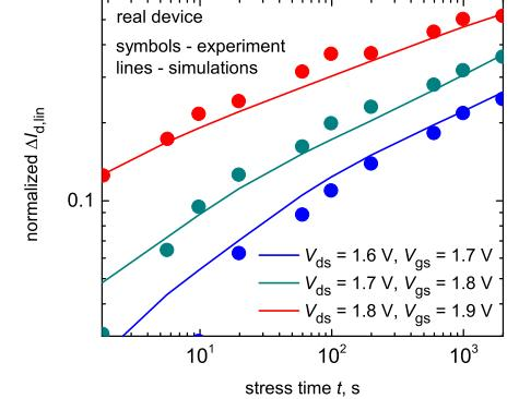
Figure 5: Measured and simulated  $\Delta I_{d,lin}(t)$  traces for three stress conditions show very good agreement.
