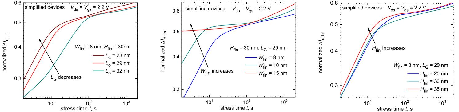
Figure 11:  $\Delta I_{d,lin}(t)$  traces simulated for three different series of devices (with varying  $L_G$ ,  $W_{fin}$ , and  $H_{fin}$ ) for  $V_{ds} = V_{gs} = 2.2$  V.
