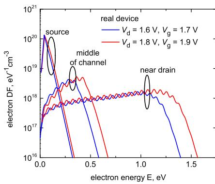
Figure 2: Electron DFs calculated for two combinations of  $V_{gs}$ ,  $V_{ds}$ , at the edge between the sidewall and the top of the fin for three different positions: at the source, in the middle of the channel, and at the drain.
