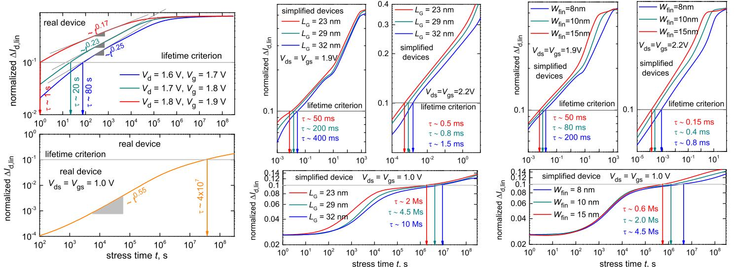
Figure 12:  $\Delta I_{d,lin}(t)$  dependences calculated for the real device and two series (with varying  $L_G$  and  $W_{fin}$ ;  $H_{fin}$  effects HCD insignificantly and corresponding data are not shown here) of simplified FinFETs. Data for stress conditions and for bias close to the operating voltage ( $V_{ds} = V_{gs} = 1.0$  V) are plotted. In order to enable extraction of the device lifetime, these traces are obtained also for shorter stress times as compared to Figs. 9, 11.
