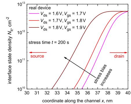
Figure 3: The  $N_{it}$  density throughout the fin/dielectric interface of the real device for  $V_{ds} = 1.7$  V,  $V_{gs} = 1.8$  V and  $t \sim 200$  s.
