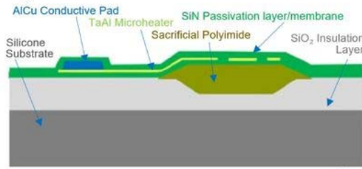
Figure 1: Two-dimensional cross section cut through the material stack making up the micro-heater. The primary materials are shown, including the sacrificial Polyimide, which, when removed, forms the air cavity and the suspended membrane, ensuring thermal isolation between the membrane micro-heater and the underlying Si wafer.
