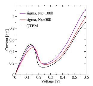
Fig. 3: The numerical solutions of the constrained sigma equation change with grid refinement, but they are quite stable. The resonance from the quantum transmitting boundary method (QTBM) is reproduced.
