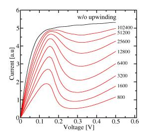
Fig. 2: Breakdown of Frensley's Method. The upper black line is the numerical solution of the unconstrained sigma equation (anti-periodic BCs) without upwinding. The red lines are I–V curves obtained with Frensley's discretization using upwinding. The grid is refined from Nx=800 up to Nx=102400.
