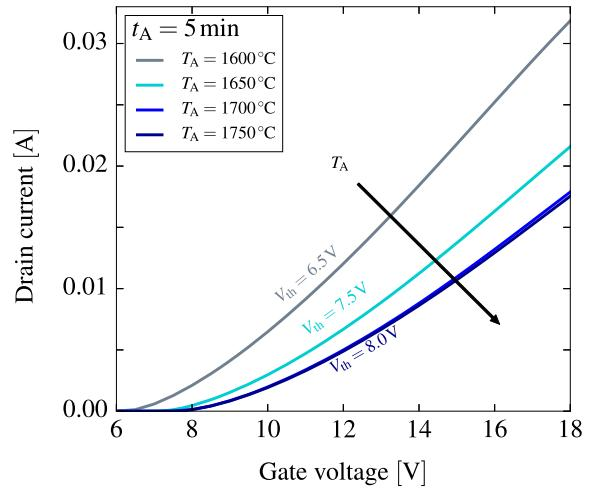
**Fig. 6.** Transfer characteristics for different annealing temperatures. Elevated annealing temperatures result in higher electrically active Al concentration in the channel, which causes a threshold voltage shift.
