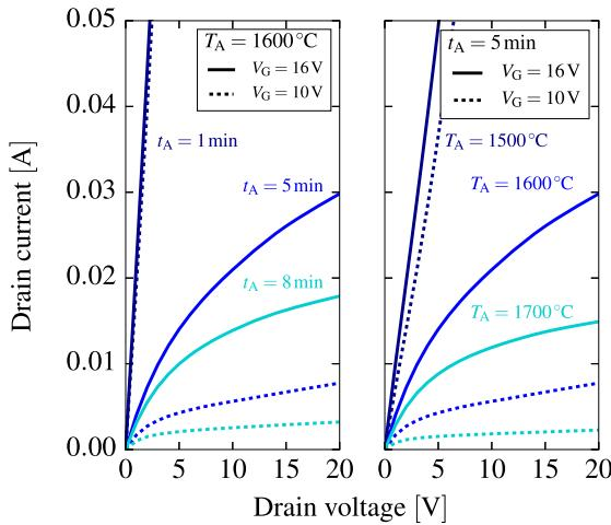
**Fig. 5.** Output characteristics for various annealing times (temperatures) for  $T_A = 1600 \text{ }^\circ\text{C}$  ( $t_A = 5 \text{ min}$ ). The output characteristics are very sensitive to the annealing variables, which is a consequence of a shift of the threshold voltage (see also Fig. 7). In addition, two annealing configurations which result in purely resistive behavior are shown. In these cases, the active acceptor concentration is insufficient to form the n-p-n sequence.
