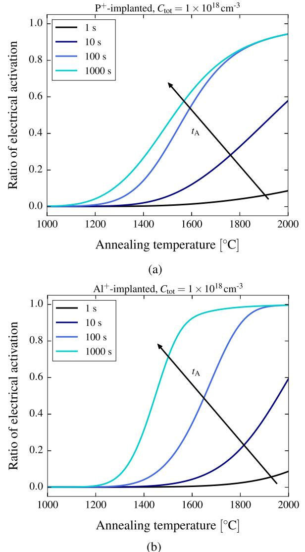
**Fig. 1.** Ratio of electrical activation as predicted by the transient annealing models (1) and (2) for (a) P- and (b) Al-implanted 4H-SiC as function of annealing temperatures for different annealing times. For both species, a total implanted concentration  $C_{\text{tot}} = 10^{18} \text{ cm}^{-3}$  is assumed.
