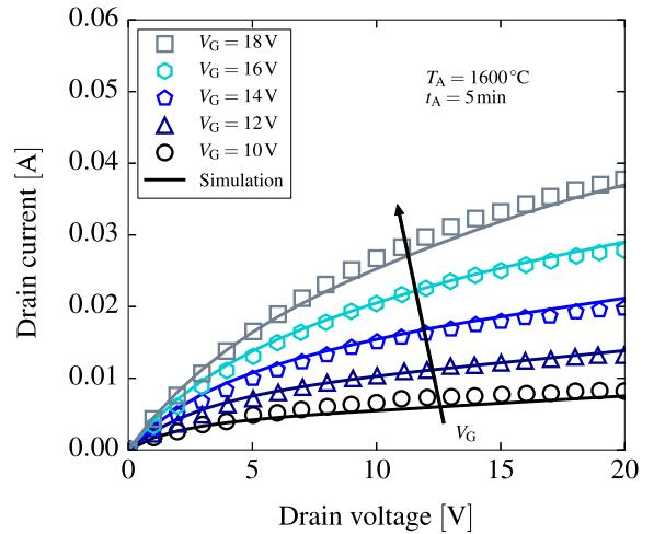
**Fig. 4.** Simulated and experimentally observed DMOSFET output characteristics for the annealing process parameters and device geometry as presented by Saha and Cooper [19]. The simulations accurately reproduce the experimentally obtained characteristics for any given gate voltage from 10 to 18 V.
