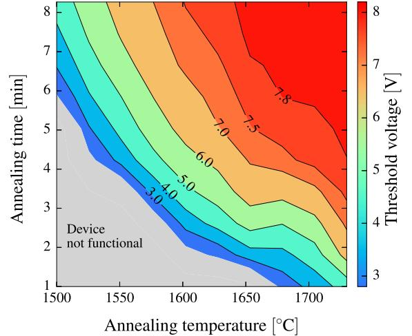
**Fig. 7.** Phase diagram of the threshold voltage as a function of annealing temperature and annealing time. The gray region is the phase space of the annealing variables which result in nonfunctional devices.
