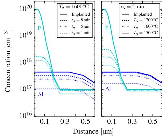
Fig. 3. Doping profiles for various annealing times (temperatures) for  $T_A = 1600^\circ\text{C}$  ( $t_A = 5$  min). Solid (dashed) lines: implanted (electrically active) doping profile. Due to the high-implanted P concentrations, the activation efficiency is strongly limited by the annealing temperature. For the implanted Al dopants, this is not the case, because the total implanted concentration is two orders of magnitude lower.
