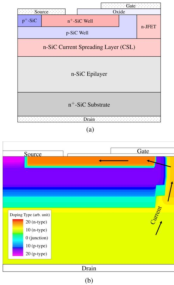
Fig. 2. (a) Schematic cross section of the examined 4H-SiC DMOSFET. This vertical power device is fabricated by implanting Al (p-type) and P (n-type) into an n-doped epitaxial layer. (b) Cross section of the device structure after process simulation, illustrated with the net concentration of implanted dopants. Arrow: path of the conduction current.
