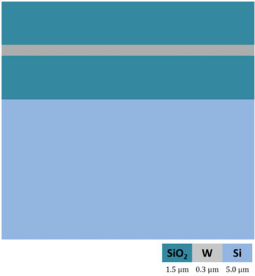
Fig. 2.20 Example for a thin film stack for numerical determination of the crack driving force
