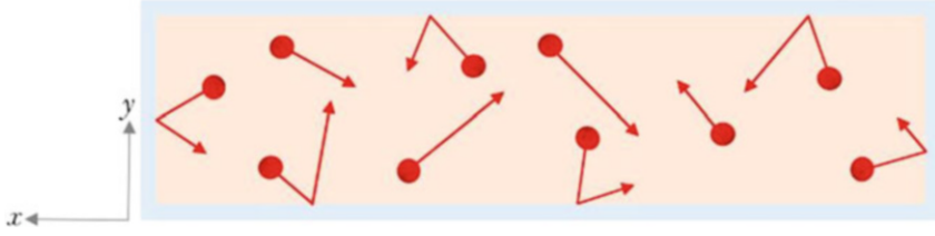
Fig. 2.5 Phonon trajectories in a silicon dioxide thin film with boundary effects
