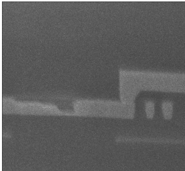
Figure 7: FIB cross-section of interconnect after an electromigration test [13] (courtesy of Dr. Lucile Arnould).
