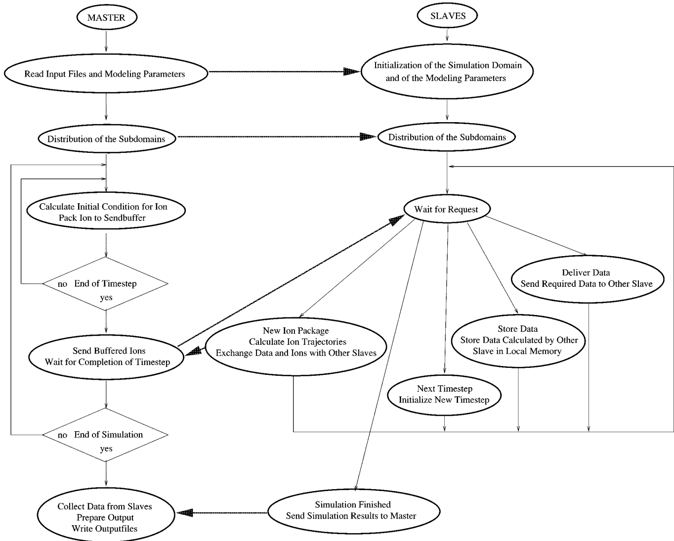
Fig. 5. Schematic description of the simulation flow of the master process and of a slave process. The thick arrows denote communication events between the master and the slave.
