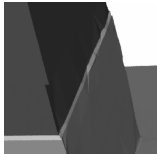
Fig. 10. Detailed view "1" of Fig. 9. The picture shows the under etching of nitride and oxide that takes place due to the imperfect anisotropy of the etching process. The different etching rates that apply to silicon, oxide, and nitride are visible.
