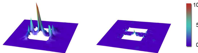
Fig. 3. Left: resulting error norm without mesh refinement. Right: error norm after three mesh adaptation steps. The error values are distributed between 10, which means a high local error norm and 0, which means a low local error norm.
