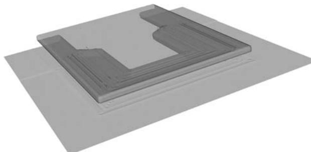
**Fig. 6** During the etching process, the isolators are attacked. Material Iso1 has nearly twice the etch speed than Iso2
