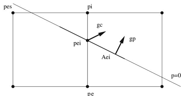
**Fig. 1** Two-dimensional discretization of the etcher/material interface. The level-set  $\Phi = 0$  intersects at  $p_{ei}$  between the grid points  $p_e$  inside the etcher atmosphere and  $p_i$  inside the solid. Characteristic parameters of the discretization are the gradient of the etcher front  $\nabla \Phi$ , the gradient of the etchant concentration distribution  $\nabla c$ , and the assigned interface area  $A_{ei}$
