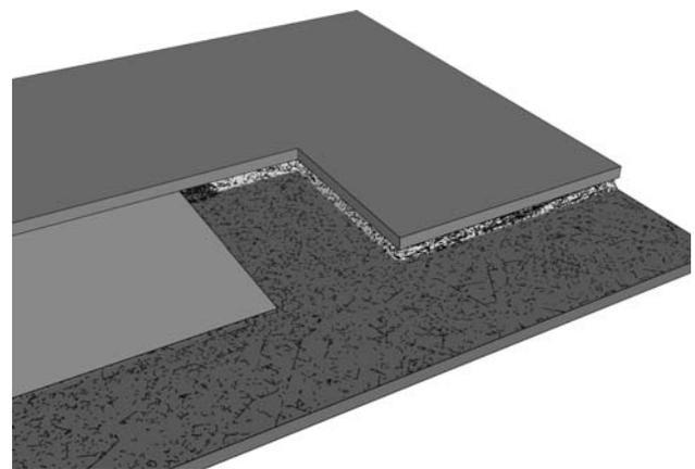
**Fig. 8** Situation after reaching final time, the level-set representation is back-converted to a tetrahedral representation.  $\text{SiO}_2$  has been removed and the Poly is free standing. Clear underetch of the PECVD layer under the Poly layer can be seen
