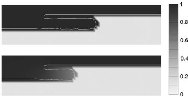
**Fig. 2** Comparison of the etch front after a simulation with neglect and inclusion of diffusive transport
