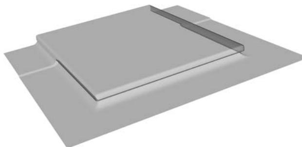
**Fig. 5** The etching process started. First the former planar surfaces on top of the isolators are etched away
