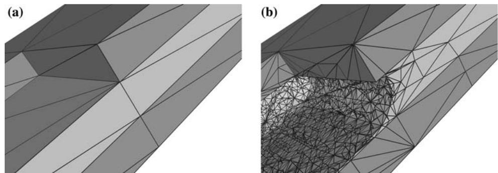
**Fig. 4** Original material constellation on a tetrahedral mesh. The materials Iso1 and Iso2 are etched away
