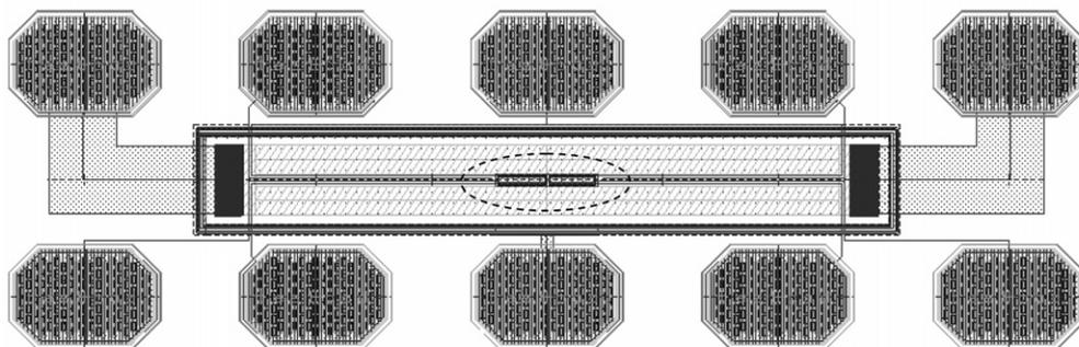
Fig. 1. Device embedded into polyheater structure. The transistor is pointed out by the circle.
