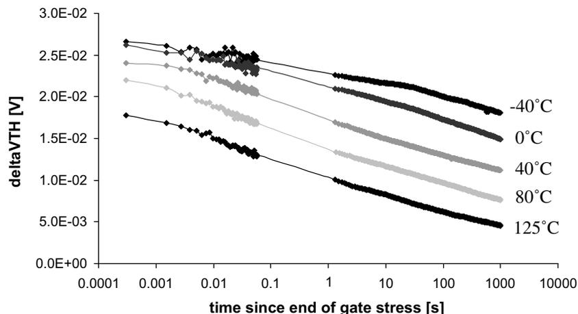
Fig. 3. Recovery of threshold voltage stress conditions: VGS = –16.5 V, VDS=0.0 V, T = 125 °C; recovery conditions: VGR = –1.1 V, VDR = –2.5 V, T = –40/0/40/80/125 °C.
