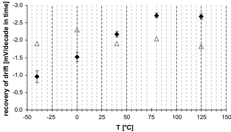
Fig. 4. Temperature dependent recovery  $\blacklozenge$  between 1 ms and 100 ms post stress  $\triangle$  between 10 s and 1000 s post stress.
