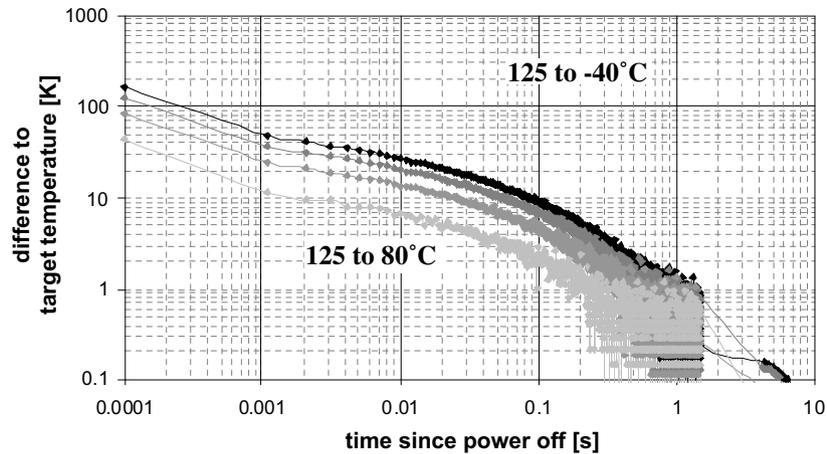
Fig. 2. Temperature characteristics of the polyheater during cooling from stress temperature (125 °C) to different recovery target temperatures (–40/0/40/80 °C).
