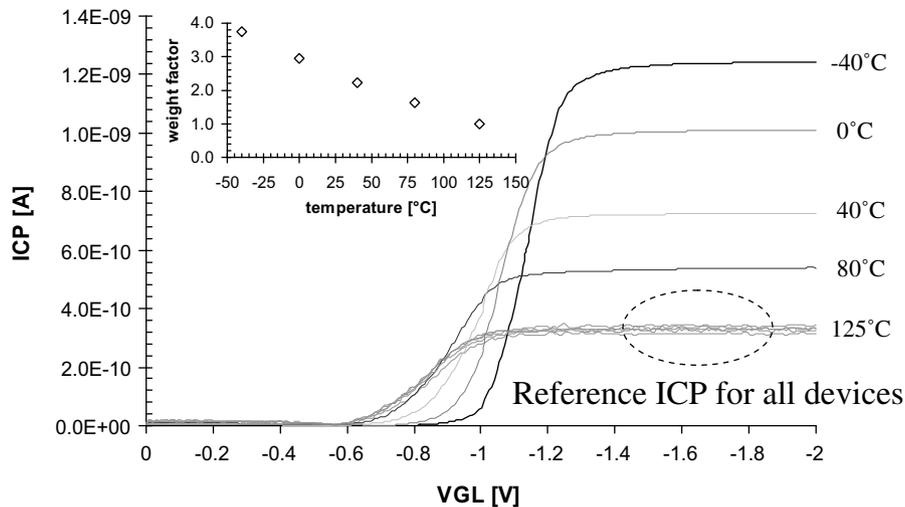
Fig. 7. Virgin CP currents measured at different recovery temperatures and at stress temperature. The illustration in the left corner shows the evaluated weight factors  $w(T_{ri}, T_s)$ .
