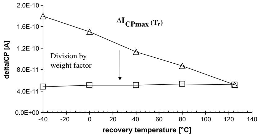
Fig. 5. Increase of CP current after stress and recovery while the triangles reflect the pure difference of  $\Delta I_{CP,max}(T_r)$ , the squares show the difference corrected by the temperature weighting factor.
