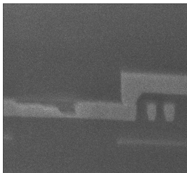
Fig. 11. FIB cross section of interconnect after an electromigration test [18] (courtesy of Dr. Lucille Arnaud).
