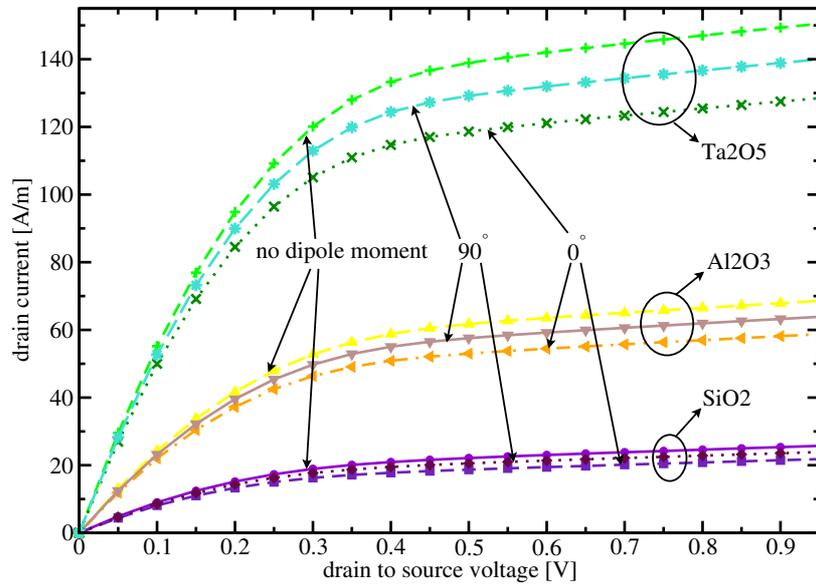
**Fig. 8.** Output curves for  $\text{SiO}_2$ ,  $\text{Al}_2\text{O}_3$ , and  $\text{Ta}_2\text{O}_5$  for calculation without dipole moment, angle  $0^\circ$  (perpendicular to surface), and angle  $90^\circ$  (parallel to surface).
