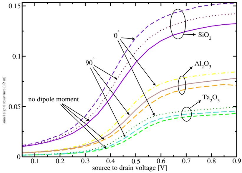
**Fig. 10.** Small signal resistance for SiO<sub>2</sub>, Al<sub>2</sub>O<sub>3</sub>, and Ta<sub>2</sub>O<sub>5</sub> calculated without dipole moment, angle 0° (perpendicular to surface), and angle 90° (parallel to surface) at bound state (biotin-streptavidin) for 10 nm average distance.
