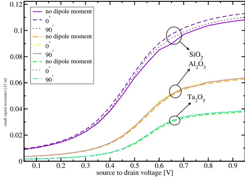
**Fig. 9.** Small signal resistance for SiO<sub>2</sub>, Al<sub>2</sub>O<sub>3</sub>, and Ta<sub>2</sub>O<sub>5</sub> calculated without dipole moment, angle 0° (perpendicular to surface), and angle 90° (parallel to surface) at biotin only.
