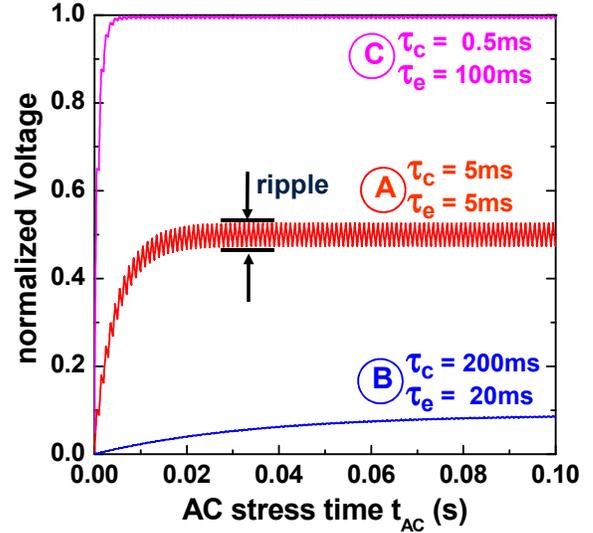
Figure 2: Some examples of charging curves of RC-elements (=defects) with different charging time constants  $\bar{\tau}$  (eq. 3) and different ratios  $\tau_c/\tau_e$ , B=0.1, A=1, C=20. Duty factor is 50% for all curves.
