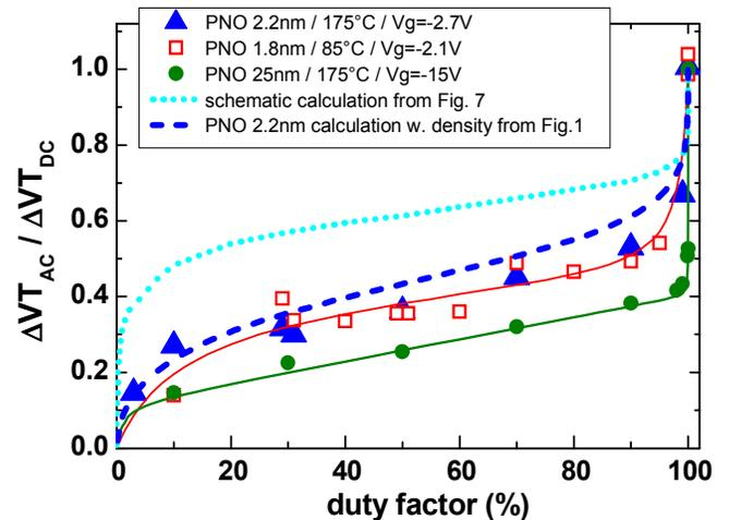
Figure 6. Experimental and calculated curves  $\Delta VT$  vs duty factor. The calculated curve for the PNO is from the model Fig. 1b and is in fair agreement to experiment. The "schematic" calculation is from an integration over the occupied areas in Fig. 7. All data are for  $f=100$  kHz and a measuring delay of 1  $\mu$ s after completion of a stress phase.
