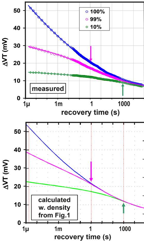
Figure 9 Measured and calculated recovery after stress with duty cycle 100% / 99% / 10%. The corresponding stress times  $t_{AC}$  were 100s / 101s / 1000s so that the *net stress times*  $t_{AC} \times \beta$  are the same for all 3 curves. Arrows mark the points where the AC recovery curves are supposed to merge with the DC curve (emp. green arrows Fig. 4).
