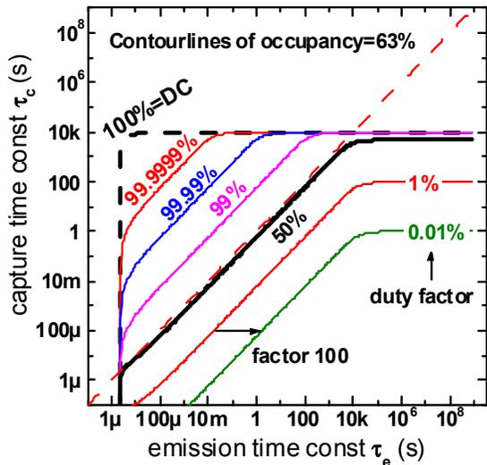
Figure 7. Calculated contour lines of an  $(1-e)$  occupancy level in the  $\tau_e$ - $\tau_c$  plane after AC-stress with the duty factor as parameter. Stress frequency is 100 kHz, stress time is 10 ks and measuring delay is 1  $\mu$ s. For a "flat" spectral defect density the  $\Delta VT$  corresponds to the area enclosed by the contour lines.
