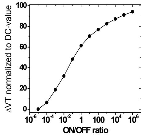
Figure 8. Calculated  $\Delta VT$  calculated just from integrating over the occupied area in Fig. 7. This curve is identical to the "schematic" curve in Fig. 6. To avoid a divergent integral the area in Fig. 7 has been clipped for values  $\tau_e > \tau_e * 10^5$ . The transformation from duty factor to ON/OFF ratio converts any S-shaped curves into an almost linear curve and vice versa.
