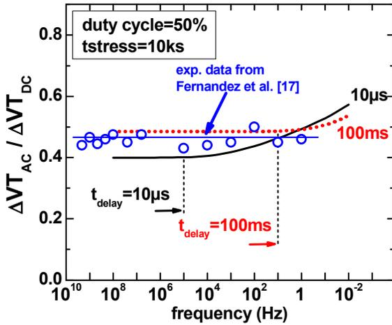
Figure 5: Frequency dependence, calculated with the model parameters from Fig. 1b in comparison with experimental data from ref.[17]. The experimental data were taken with a measuring delay  $t_D=10$  s; the calculations have been done with  $t_D=10$   $\mu$ s and 100 ms (see right hand labels). The frequency dependence vanishes for frequencies  $f > 1/t_D$ .
