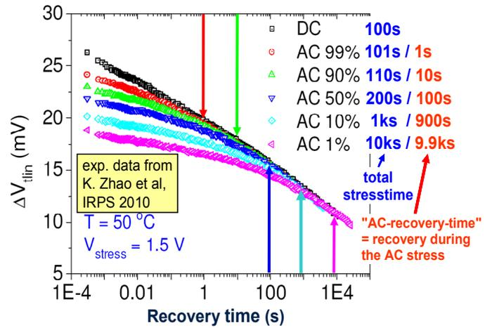
Figure 10. Recovery curves all taken after a net stress time of 100 s with various duty factors. The arrows mark the position where the AC-curves and the DC-curve (100%) are expected to merge.
