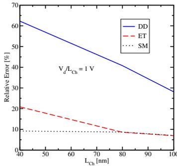
**Fig. 5.** Relative error of the current computed with macroscopic transport models. While the drift-diffusion and the energy-transport models are gradually losing their validity with the channel length reduced, the six moments model maintains its accuracy down to the channel length of 40 nm.
