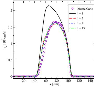
**Fig. 1.** Average velocity along the *nin* structure computed by solving the Boltzmann transport equation with the Monte Carlo method and using the spherical harmonic expansion method, with different numbers of terms included in the series (1). It is demonstrated that even in a short-channel structure the series expansion with terms only up to  $l = 9$  included provides excellent results as compared to the more time consuming Monte Carlo data.
