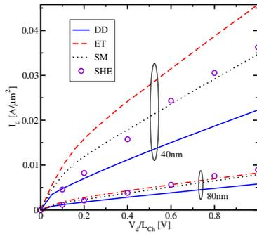
**Fig. 3.** The same as in Fig. 2 for shorter devices. The six moments model gives results closest to the results of Monte Carlo and the spherical Harmonic expansion methods.
