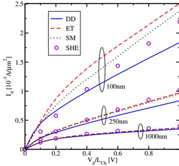
**Fig. 2.** Current-voltage characteristics for devices with different channel length computed with the spherical harmonic expansion method and using macroscopic transport models based on moments of the distribution function. Here DD stands for the drift-diffusion model, ET for energy-transport model, SM for the six moments model, and SHE for spherical harmonic expansion.
