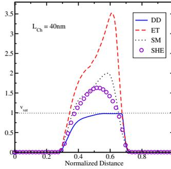
**Fig. 4.** Average velocity along the device with 40 nm channel length computed with the macroscopic transport models and with the spherical harmonic expansion method (equivalent to the Monte Carlo results). While the drift-diffusion model underestimates the velocity and current, the energy-transport model overestimates the velocity in short-channel devices. The six moments model improves the situation.
