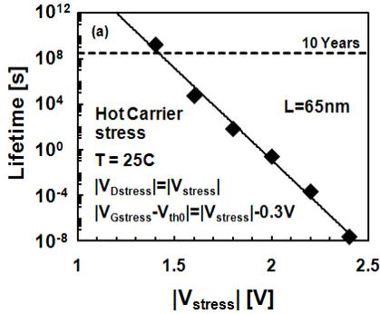
Fig. 6: Hot Carrier Injection (a) and Time Dependent Dielectric Breakdown (b) do not constitute a showstopper for our optimized SiGe device. In particular, < 6 soft breakdowns per chip (Area=0.1cm<sup>2</sup>) can be expected during application lifetime at  $V_{DD}=1V$  (inset documents extrapolation of TDDB data).
