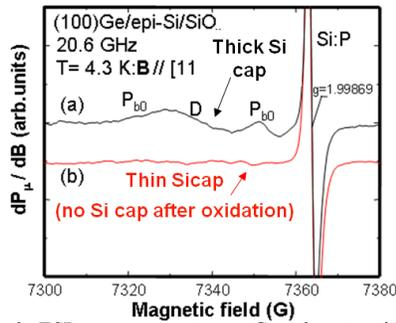
**Fig. 9:** ESR measurement on a Ge substrate with a thick Si cap top revealed a high  $P_{b0}$  density ( $\sim 1 \times 10^{12} \text{ cm}^{-2}$ ) while these defects could not be detected ( $< 10^{11} \text{ cm}^{-2}$ ) for a very thin and almost completely oxidized Si cap.
