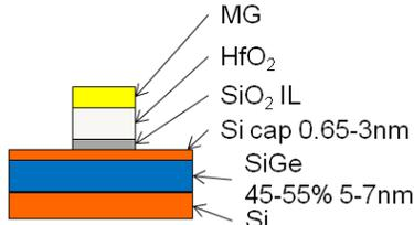
Fig. 1: Gate-stack sketch of the SiGe device.
