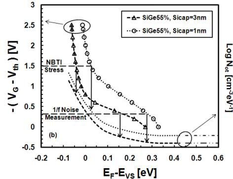
**Fig. 12:** (a, left) A clear correlation between the initial  $V_{th0}$  and  $\Delta V_{th}$  during NBTI stress was consistently observed on our SiGe devices with different gate-stacks: devices with lower initial  $V_{th0}$  always showed reduced  $V_{th}$  instability, at any given stress condition ( $|V_{Gstress} - V_{th0}|$ ). (b, right) This remarkable trend can be explained with the model proposed in Fig. 11.
