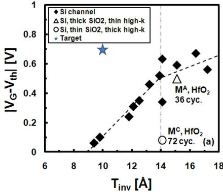
Fig. 4: Similar  $T_{inv}$  was obtained on a Si ref. device with thin HfO<sub>2</sub> + weak scavenging ( $M^A$ ) and with thick HfO<sub>2</sub> + aggressive scavenging ( $M^C$ ). IL scavenging is shown to reduce NBTI reliability remarkably more than high-k scaling.
