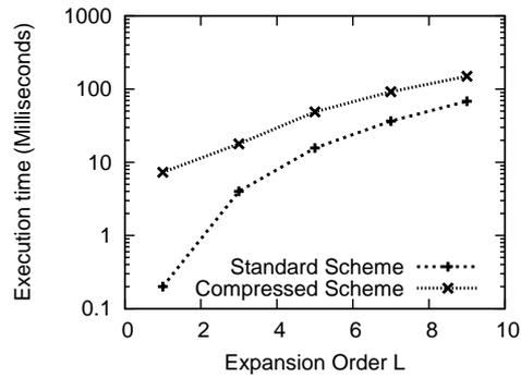
dimensional device simulations especially for larger expansion orders  $L$ . On a single CPU core, the small price to pay is a runtime penalty on matrix-vector multiplication of about a factor of two. However, the proposed method is expected to outperform the traditional storage scheme on parallel architectures.
