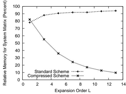
ments for the full simulation is still  $\mathcal{O}(NL^2)$ , but the constant of proportionality is of order one, while for the full system matrix it is around  $11C_{\text{sparse}} \approx 100$ , so a reduction of memory requirements by two orders of magnitude is obtained.
