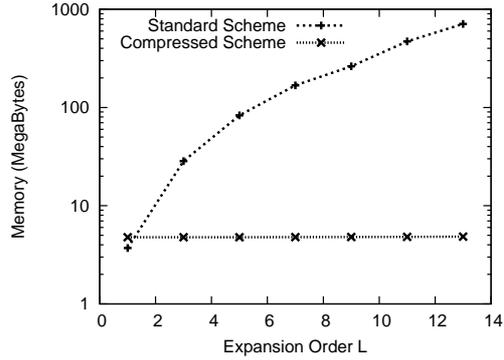
**Fig. 2** Memory used for the system matrix in relation to the total amount of memory used (i.e. system matrix, unknowns and right hand side).
