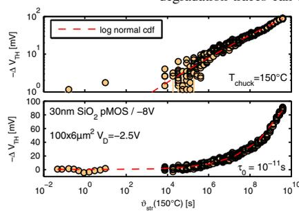
Fig. 17. The temperature-time concept makes it possible to access the degradation of power devices at use conditions. Depicted is an example of such a measurement where the degradation at -8V gate bias was achieved by accelerating with 300°C. We remark that based on the results in this paper, temperature acceleration is a far more promising approach to access lifetime data compared to conventional downscaling from large stress oxide fields.
