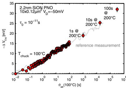
Fig. 13. Switching the device temperature to a higher value during stress accelerates the degradation. For small temperature switches, the correct interpretation of the acceleration can be demonstrated by a comparison with long-term OTF data (reference measurement).
