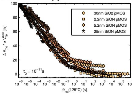
Fig. 4. The experiment of Fig. 3 was repeated on several different technologies with different gate dielectrics ( $\text{SiO}_2$  and PNO SiON) and different gate oxide thicknesses. The temperature-time concept works for all observed technologies with one single value of  $\tau_0$ . The graph was normalized to the maximum drift 10ms post stress at  $-60^\circ\text{C}$ .
