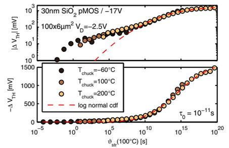
Fig. 12. In Fig. 11 we accelerated the test using one temperature and increasing stress times. Now, we always used 10s of stress but with increasing temperatures from  $T_{chuck}$  to the maximum achievable temperature with the poly-heater (upper plot of Fig. 8).
