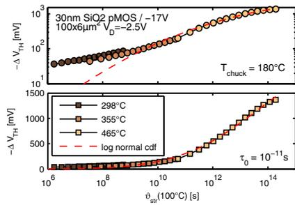
Fig. 11. Temperature accelerated interrupted stress measurements may also be performed on devices having 30nm SiO<sub>2</sub> gate oxides. Again, long-term high-temperature data can be perfectly fitted by a log-normal distribution.
