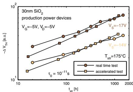
Fig. 16. Long-term NBTI degradation data of state-of-the-art power pMOS devices (gathered over several months) are reproduced within less than a day by using temperature accelerated testing with the poly-heater. Considering the vastly different measurement methods used for the reference data, which included large (manual) delay times, which could only be roughly emulated by the poly-heater technique, the agreement is satisfactory.
