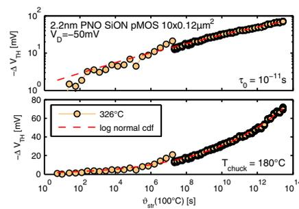
Fig. 14. Temperature accelerated OTF degradation data shows the same behavior as the data from interrupted stress measurements. Again, the saturation of the power law can be perfectly matched by a log-normal distribution of capture time constants.
