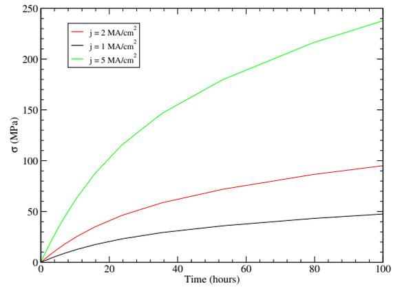
Fig. 3. Hydrostatic stress build-up as a function of time.
