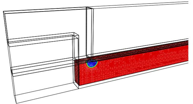
Fig. 4. Order parameter separating the bulk (red), the void (blue), and the diffuse interface region.
