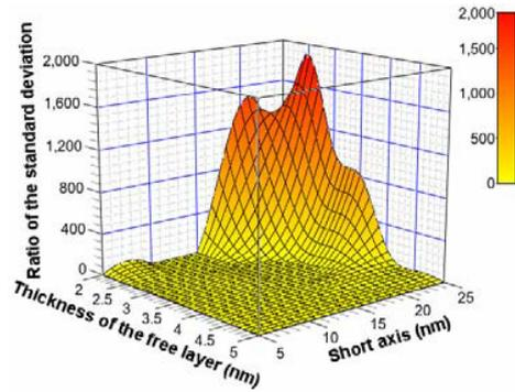
Figure 8. Ratio of the standard deviation of the switching time in the monolithic structure and composite structure as function of thickness of the free layer and short axis length. The long axis is fixed at 52.5nm and the thickness of the fixed layers are 10nm.
