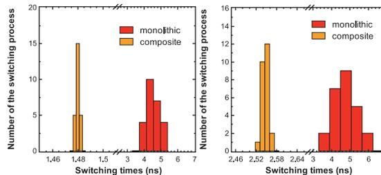
Figure 2. Distributions of the switching times for an MTJ of  $75 \times 25 \text{ nm}^2$  (left) and  $155 \times 60 \text{ nm}^2$  (right) cross-section with monolithic and composite free layer.
