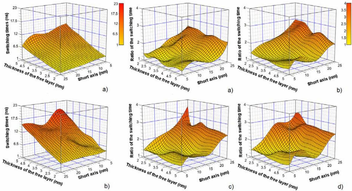
Figure 6. Switching times in the composite structure (a) and monolithic structure (b) as function of thickness of the free layer and short axis length. The long axis is fixed at 52.5nm and the thickness of the fixed layers are 5nm.
