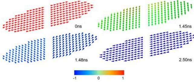
Figure 4. Snapshots of the switching process for an MTJ with a composite free layer with dimensions  $75 \times 25 \text{nm}^2$ . The direction of the magnetization is shown by unit vectors, color indicates the value of the  $x$ -component of magnetization, the  $x$ -axis is directed along the long axis of the ellipse.
