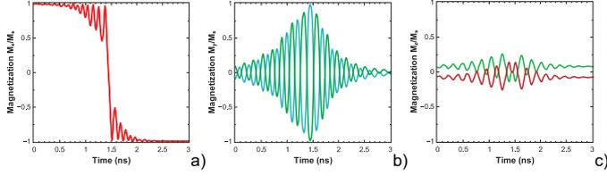
Figure 3. Magnetization components as a function of time for an MTJ element of  $75 \times 25 \text{nm}^2$  with a composite free layer. The magnetization of the left and right half is shown separately.
