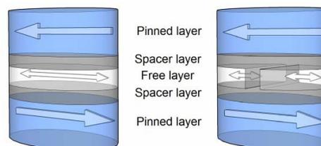
Figure 1. Schematic illustration of penta-layer MTJs with monolithic (left) and composite free layer (right).
