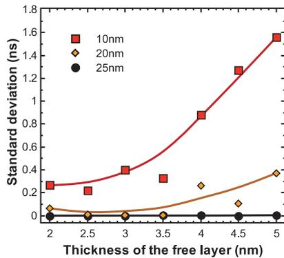
Figure 9. The standard deviation of the switching time distribution in the composite structure as a function of thickness of the free layer. The long axis is fixed at 52.5nm and the thickness of the fixed layers are 15nm. Dependences are shown for the short axis of 10nm, 20nm, and 25nm.
